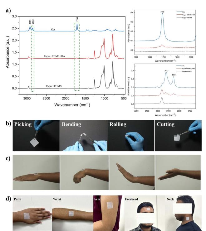
Fig. 2 (a) ATR-FTIR spectra of the developed adhesive patch and its expanded view. (b) Photographs showing its excellent adhesion properties towards different materials. (c) Photographs showing the excellent mechanical flexibility of the prepared wearable adhesive patch. (d) Photograph of the wearable patch showing strong adherence to human skin, even during dynamic wrist movements.
