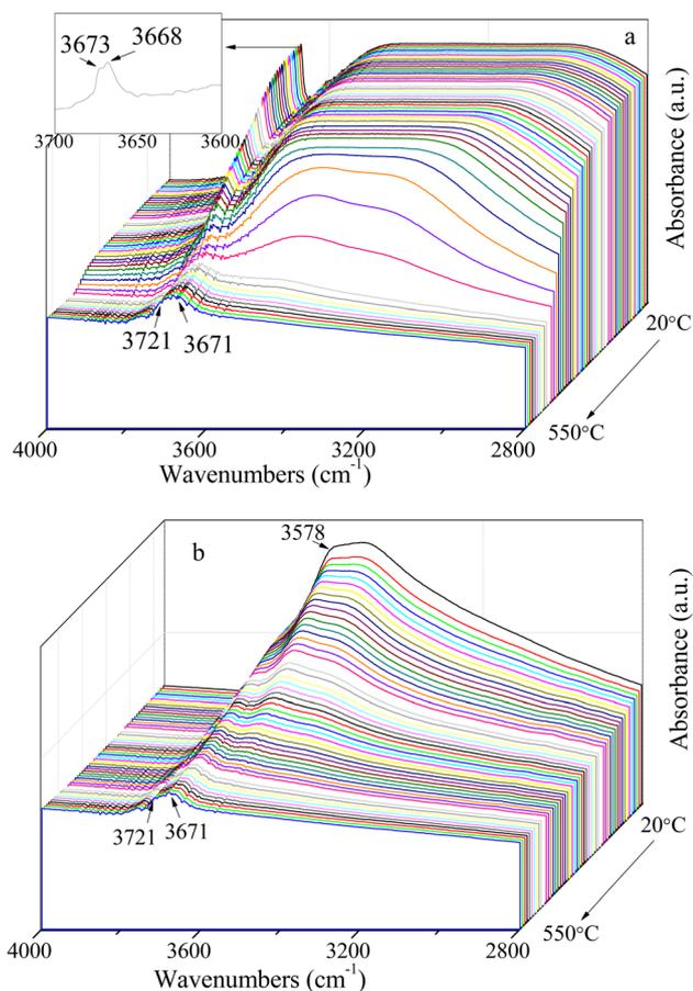
Fig. 7 Change of IR spectra (OH region) of the Au/ $\gamma$ -ALOOH (a) and Au/ $\gamma$ -Al<sub>2</sub>O<sub>3</sub> (b) as a function of temperature.
