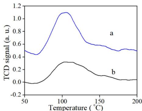
Fig. 6 CO<sub>2</sub>-TPD profiles of Au/ $\gamma$ -ALOOH (a) and Au/ $\gamma$ -Al<sub>2</sub>O<sub>3</sub> (b).
