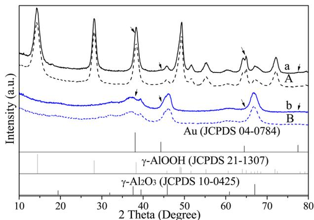
Fig. 1 Wide-angle XRD patterns of the as-synthesized  $\gamma$ -AlOOH (A, dotted line), Au/ $\gamma$ -AlOOH (a, solid line),  $\gamma$ -Al<sub>2</sub>O<sub>3</sub> (B, dotted line) and Au/ $\gamma$ -Al<sub>2</sub>O<sub>3</sub> (b, solid line). The arrows mark reflexes from Au particles.
