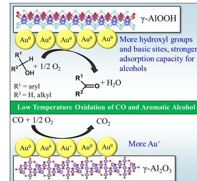
Scheme 1 Proposed reaction mechanism for the oxidation of CO and alcohol over Au/γ-AlOOH and Au/γ-Al<sub>2</sub>O<sub>3</sub> samples.
