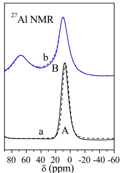
Fig. 4  $^{27}Al$  NMR spectra of as-synthesized  $\gamma$ -AlOOH (A, dotted line), Au/ $\gamma$ -AlOOH (a, solid line),  $\gamma$ -Al $_2$ O $_3$  (B, dotted line) and Au/ $\gamma$ -Al $_2$ O $_3$  (b, solid line).
