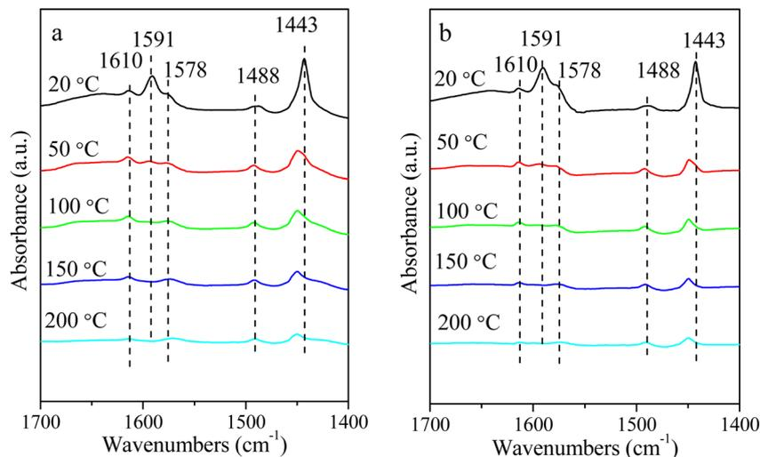
Fig. 8 IR spectra of 1-phenylethanol adsorbed on Au/γ-AlOOH (a) and Au/γ-Al<sub>2</sub>O<sub>3</sub> (b), all samples were normalized by subtracting the peak of the vacuum adsorption sample at 200 °C.
