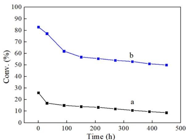
Fig. 9 The CO conversion of Au/γ-AlOOH (a) and Au/γ-Al<sub>2</sub>O<sub>3</sub> (b) samples.
