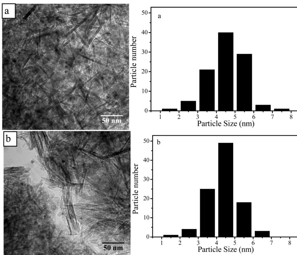
Fig. 2 TEM images (left) and Au particle size distribution (right) of the as-synthesized Au/ $\gamma$ -AlOOH (a) and Au/ $\gamma$ -Al<sub>2</sub>O<sub>3</sub> (b).
