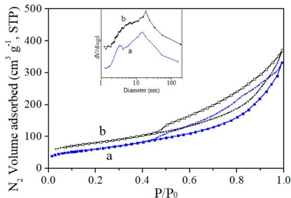
Fig. 3  $N_2$  adsorption/desorption isotherms and pore size distribution curves (insert) of the as-synthesized Au/ $\gamma$ -AlOOH (a) and Au/ $\gamma$ -Al $_2$ O $_3$  (b) samples. The curves (b) are offset a little for clarity.
