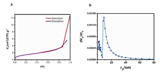
Fig. 3 Specific surface area and pore size distribution of Ag-MOF-D. Images (a) represents BET plot and (b) denotes BJH plot.
