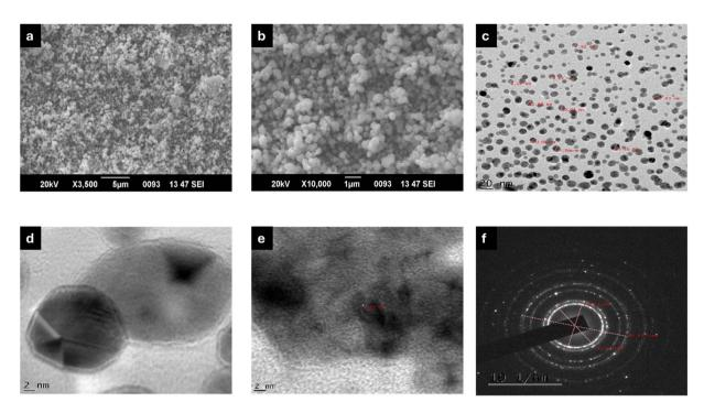
Fig. 2 Electron micrographs of Ag-MOF-D. Images (a and b) represents SEM micrographs, (c and d) demonstrates TEM micrographs, (e) exhibits lattice fringing, and (f) illustrates SAED pattern.
