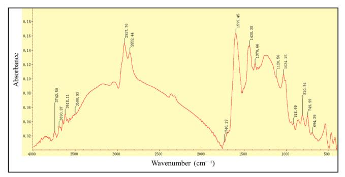
Fig. 2 Fourier transform infrared spectroscopy of coal samples at room temperature
