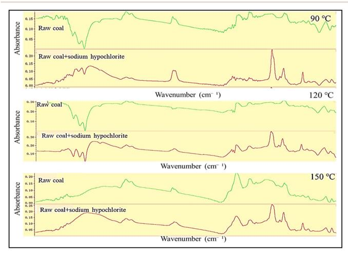
Fig. 3 Fourier transform infrared spectra of coal sample oxidation in the low temperature range: 90 °C, 120 °C, and 150 °C.
