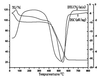
Fig. 6 Raw coal sample thermal analysis curves
