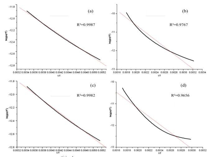
Fig. 9 Coal samples at different stages  $\ln \frac{g(\alpha)}{T} - \frac{1}{T}$ : (a) oxygen absorption weight gain stage of the raw coal sample; (c) oxygen absorption weight gain stage of the coal sample with added sodium hypophosphite; (b) thermal decomposition stages of the raw coal sample; (d) thermal decomposition stages of the coal sample with added sodium hypophosphite.
