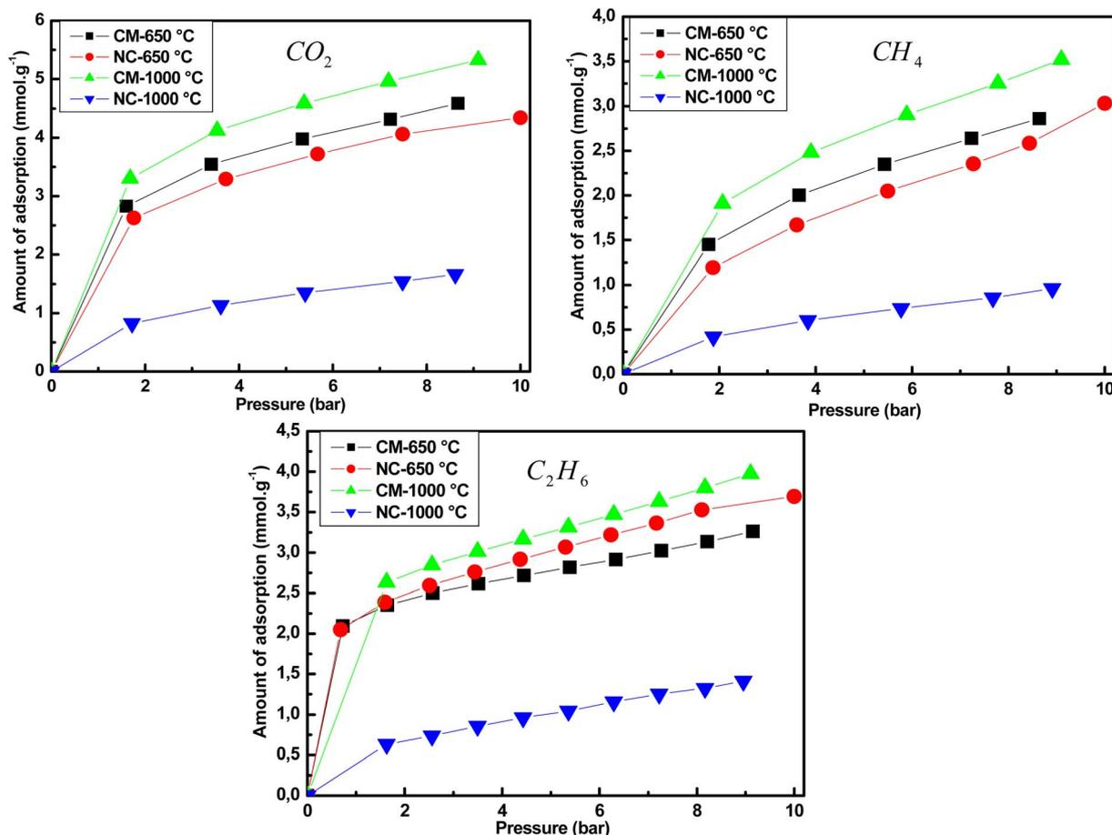
Fig. 12 Amount of adsorption of CO<sub>2</sub>, CH<sub>4</sub> and C<sub>2</sub>H<sub>6</sub> for the different samples.
