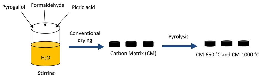
Fig. 1 Synthesis of the carbon matrix (CM).
