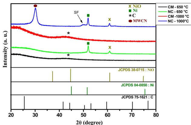
Fig. 3 X-ray diffraction of different samples.
