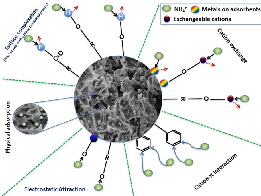
Fig. 10 Ammonium adsorption onto PWSH and PWSH@ZnO.
