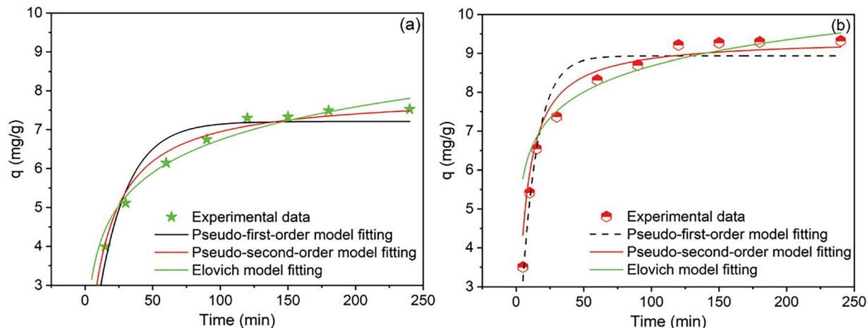
Fig. 7 Kinetic models of  $\text{NH}_4^+$  adsorption by PWSH (a) and PWSH@ZnO (b); experimental conditions: initial  $\text{NH}_4^+$  concentration  $20 \text{ mg L}^{-1}$ ; adsorbent dosage  $2 \text{ g L}^{-1}$  and pH 8.
