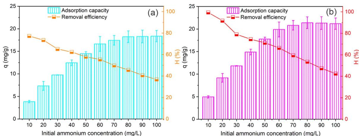
Fig. 8 Effect of  $\text{NH}_4^+$  concentration on adsorption capacity and efficiency using PWSH (a) and PWSH@ZnO (b) materials, experimental conditions: contact time of 120 min; adsorbent dosage  $2 \text{ g L}^{-1}$ , pH 8.
