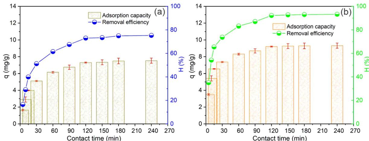
Fig. 6 Effect of contact time on the  $\text{NH}_4^+$  adsorption efficiency using PWSH (a) and PWSH@ZnO (b) materials; experimental conditions: initial  $\text{NH}_4^+$  concentration  $20 \text{ mg L}^{-1}$ ; adsorbent dosage  $2 \text{ g L}^{-1}$ , pH 8.
