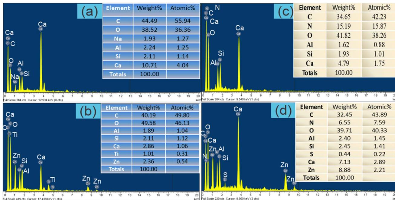
Fig. 2 EDX spectra PWSH (a), PWSH@ZnO (b), PWSH after  $\text{NH}_4^+$  adsorption (c) and PWSH@ZnO after  $\text{NH}_4^+$  adsorption (d).
