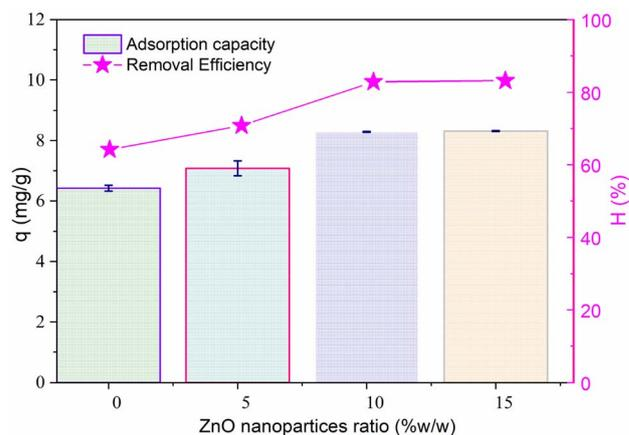
Fig. 4 The effect of the ratio of ZnO nanoparticle modification to hydrothermal paper sludge biochar (PWSH@ZnO) on  $\text{NH}_4^+$  adsorption efficiency; experimental conditions: initial  $\text{NH}_4^+$  concentration  $20 \text{ mg L}^{-1}$ , adsorbent dosage  $2 \text{ g L}^{-1}$  and pH 8, contact time of 60 min.
