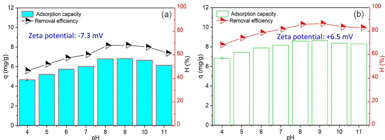
Fig. 5 The effect of pH solution on  $\text{NH}_4^+$  adsorption efficiency using PWSH (a) and PWSH@ZnO (b); experimental conditions: initial  $\text{NH}_4^+$  concentration  $20 \text{ mg L}^{-1}$ ; adsorbent dosage  $2 \text{ g L}^{-1}$ , contact time of 60 min.
