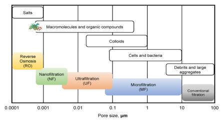
Fig. 6 Types of membrane processes and dimensions of various common pollutants.<sup>69</sup>
