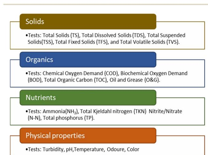
Fig. 1 Laboratory tests and analytical categories of wastewater.
