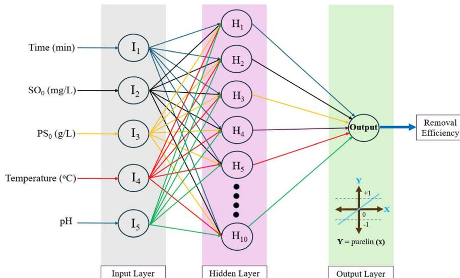
Fig. 12 The best artificial neural networks ANN topology used to predict removal efficiency of safranin O (SO) dye and optimise AOPs adapted from Fetimi *et al.*<sup>141</sup> with permission.
