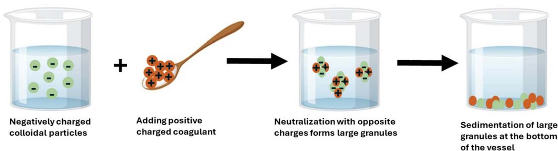
Fig. 4 Schematic diagram of the chemical coagulation mechanism.
