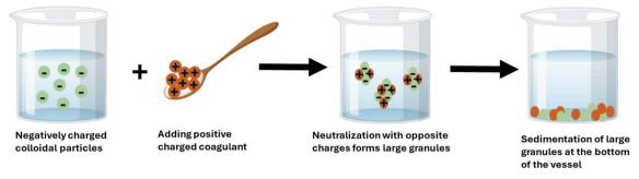
Fig. 4 Schematic diagram of the chemical coagulation mechanism.
