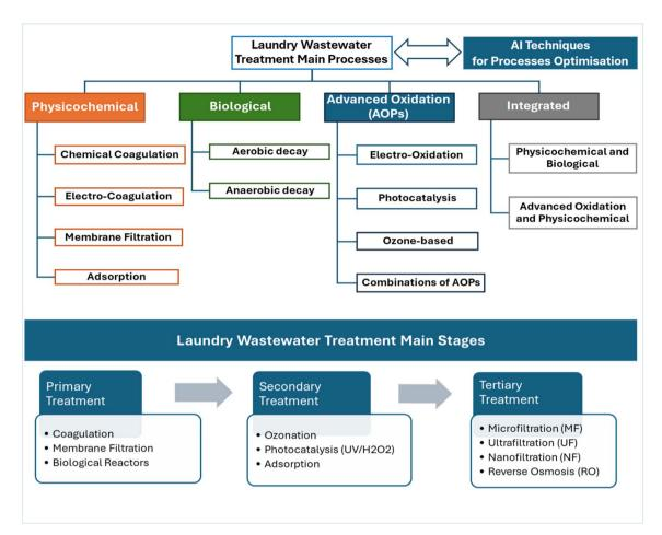
Fig. 3 Laundry wastewater treatment main processes and stages.
