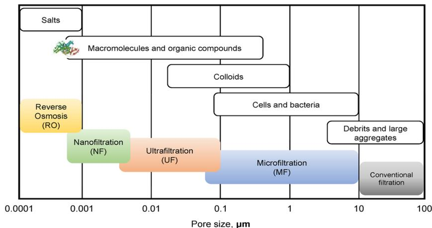
Fig. 6 Types of membrane processes and dimensions of various common pollutants.<sup>69</sup>
