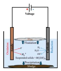
Fig. 5 Treatment mechanism of electrocoagulation process.
