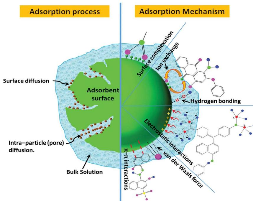
Fig. 8 Adsorption phenomenon process and mechanism.<sup>77</sup>
