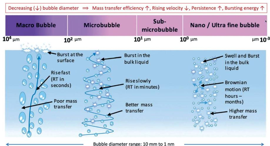
Fig. 10 Range of bubbles sizes and corresponding major properties.<sup>125</sup>
