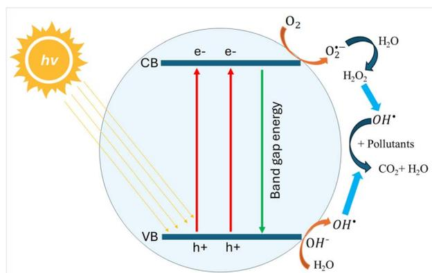
Fig. 9 Scheme of the photocatalytic degradation mechanism.
