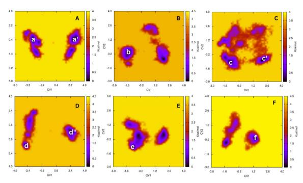
Fig. 2 FELs of six complexes AChE + compounds over equilibrium conformations via PCA approach during interval 100-200 ns of MD simulations. In particular, (A-F) patterns are FEL of compounds 12, 15, 18, 22, 25, and 26, respectively.
