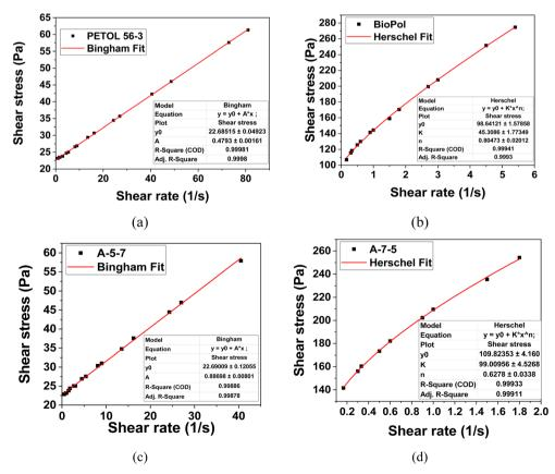
Fig. 1 The shear stress (Pa) vs. shear rate (s<sup>-1</sup>) plots of PETOL 56-3 (a). BioPol (b), component A-5-7 (c), and component A-7-5 (d).
