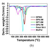
Fig. 4 (a) TG and (b) DTG profiles of polyurethane foam samples.
