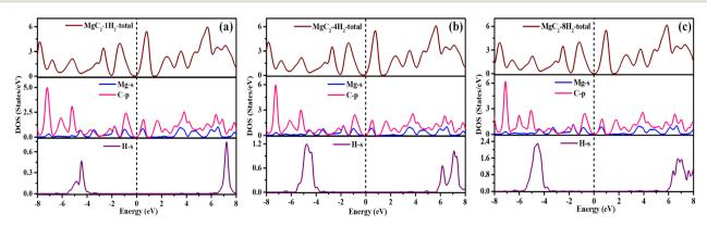
Fig. 3 DOS of (a)  $1H_2$ , (b)  $4H_2$ , (c)  $8H_2$  adsorbed MgC<sub>2</sub>.
