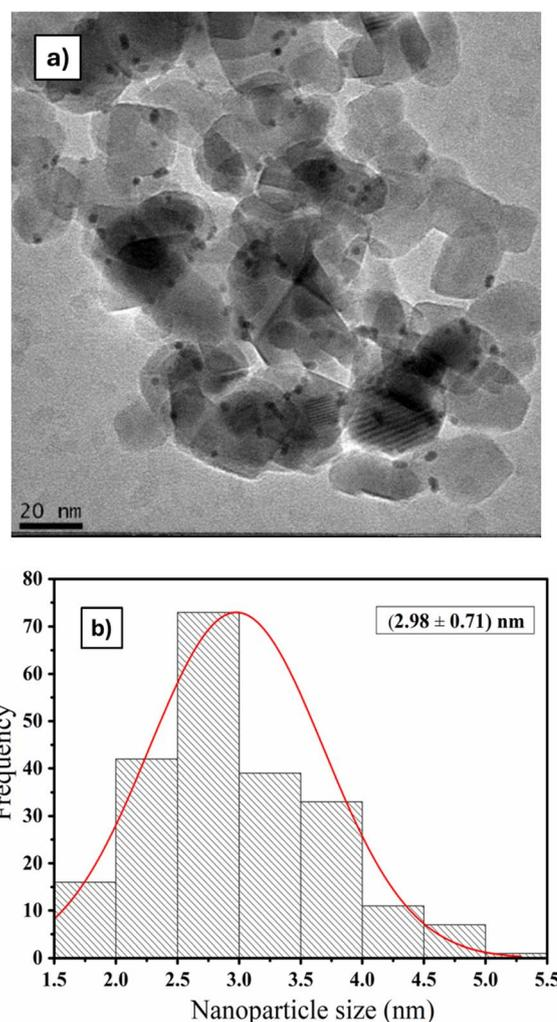
Fig. 1 (a) TEM micrograph and (b) histogram of Pt/TiO<sub>2</sub> photocatalyst.
