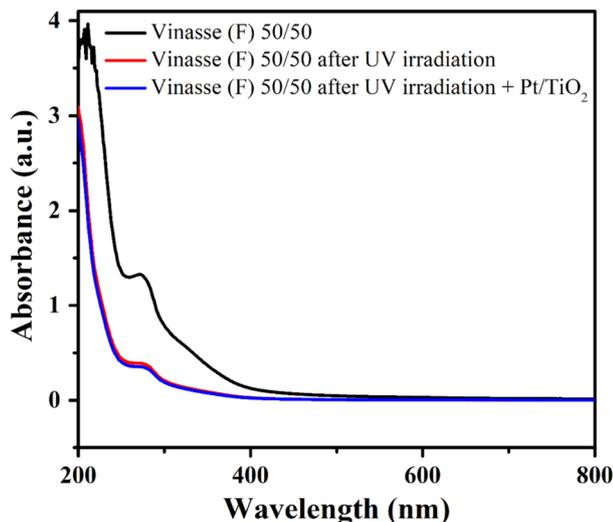
Fig. 4 UV-Vis absorption spectra of vinasse (F) SA/H<sub>2</sub>O of 50/50, after UV irradiation and after UV irradiation in the presence of Pt/TiO<sub>2</sub>.
