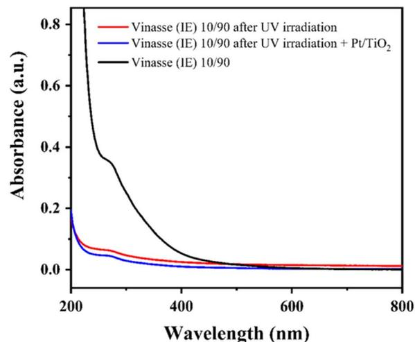
Fig. 5 UV-Vis absorption spectra of vinasse (IE) 10/90 before and after UV irradiation, and after UV irradiation in the presence of Pt/TiO<sub>2</sub>.
