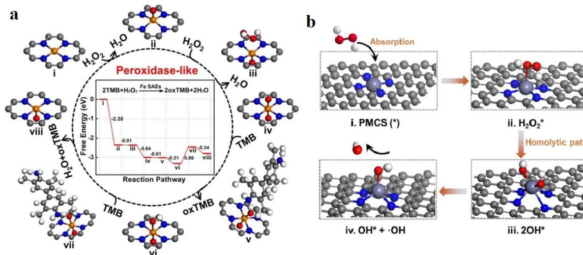
Fig. 1 (a) Diagram of the catalytic reaction procedure of the peroxidase route of SAzymes. This figure has been reproduced from ref. 40 with permission from the Royal Society of Chemistry, copyright 2019. (b) Suggested peroxidase-like catalytic performance of PMCS. This figure has been reproduced from ref. 41 with permission from Wiley, copyright 2019.
