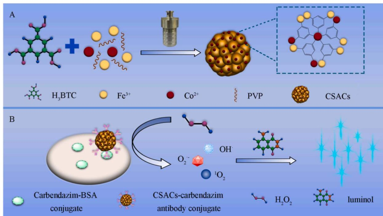
Fig. 5 (A) Solvothermal technique employed to synthesize CSACs immobilized on hybridized MOFs  $\text{Fe}_2\text{O}_3/\text{MIL-100}(\text{Fe})$ . (B) Chemiluminescent immunoassay technique used for the detection of carbendazim, with CSACs serving as signal assays. This figure has been reproduced from ref. 86 with permission from Elsevier, copyright 2022.
