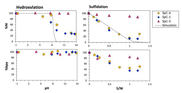
Fig. 2 Percentage of dissolved Ni and bpy in SpC-A, SpC-1, and SpC-3 during hydroxylation and sulfidation at an initial pH 3 of 4. Broken lines indicate simulated values of Ni removal as Ni(OH)<sub>2</sub> or NiS (PHREEQC version 3).
