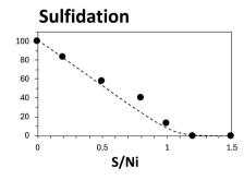
Fig. 1 Ni precipitation from SpC-0 by hydroxylation and sulfidation at an initial pH of 3–4. Broken lines indicate simulated removal as Ni(OH)<sub>2</sub> and NiS (PHREEQC version 3, Ilnl database), respectively.
