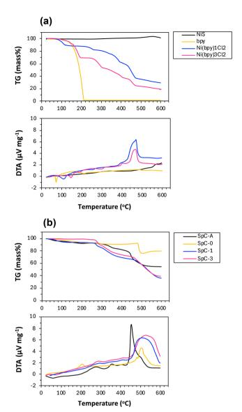
Fig. 6  $\,$  TG-DTA curves for standards (a) and Ni precipitates generated by sulfidation (b).
