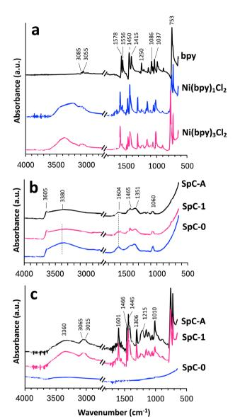
Fig. 5 ATR FT-IR spectra of standard materials (a), the hydroxide precipitates (b), and the precipitates generated by the sulfidation (c).
