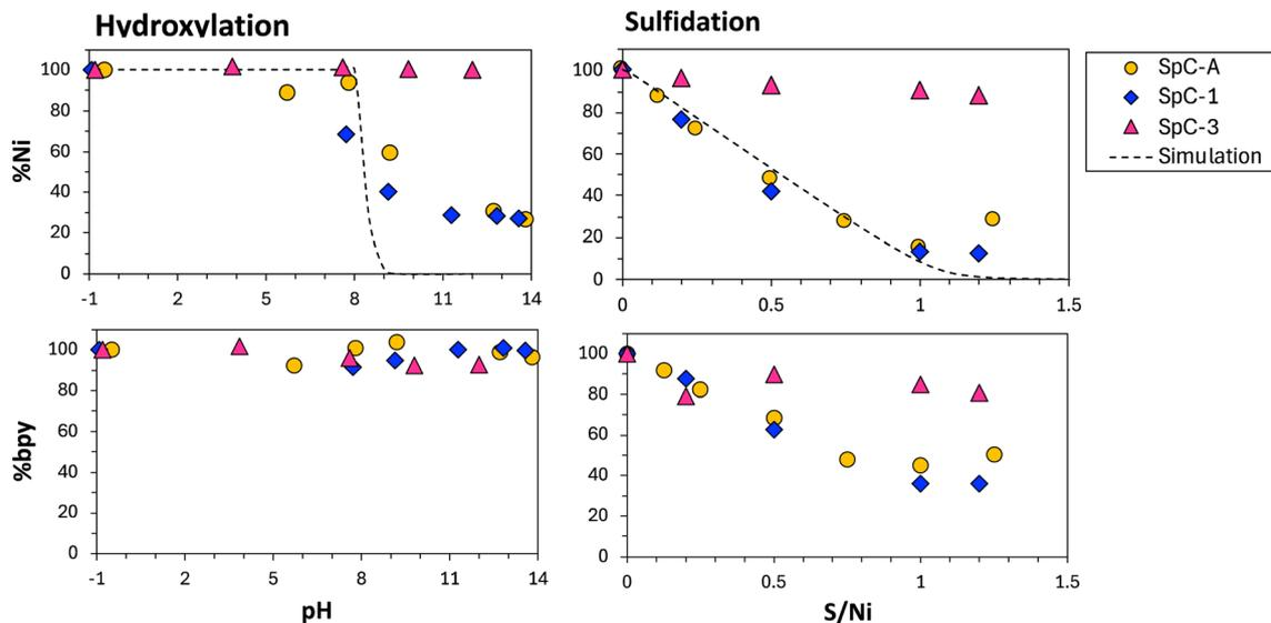
Fig. 2 Percentage of dissolved Ni and bpy in SpC-A, SpC-1, and SpC-3 during hydroxylation and sulfidation at an initial pH 3 of 4. Broken lines indicate simulated values of Ni removal as  $\text{Ni}(\text{OH})_2$  or  $\text{NiS}$  (PHREEQC version 3).
