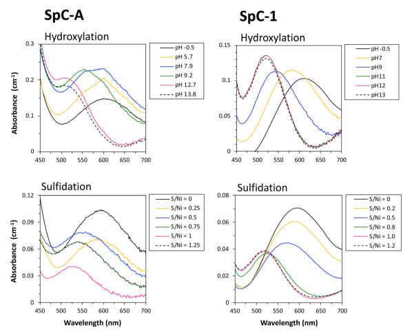
Fig. 4 Visible range absorption spectra of the SpC-A and SpC-1 filtrates ( $<0.45 \mu m$ ) after the precipitation processes.
