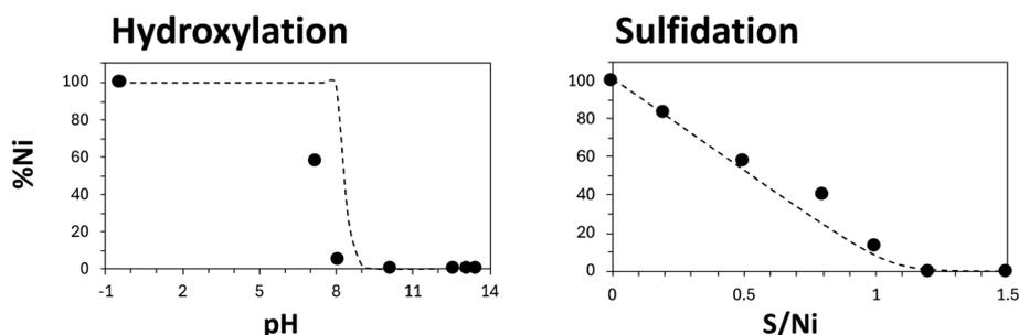
Fig. 1 Ni precipitation from SpC-0 by hydroxylation and sulfidation at an initial pH of 3–4. Broken lines indicate simulated removal as  $\text{Ni}(\text{OH})_2$  and  $\text{NiS}$  (PHREEQC version 3, llnl database), respectively.
