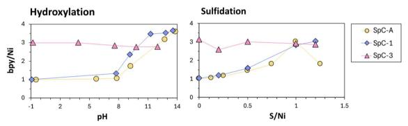
Fig. 3 Changes in the bpy/Ni molar ratio during the precipitation processes.
