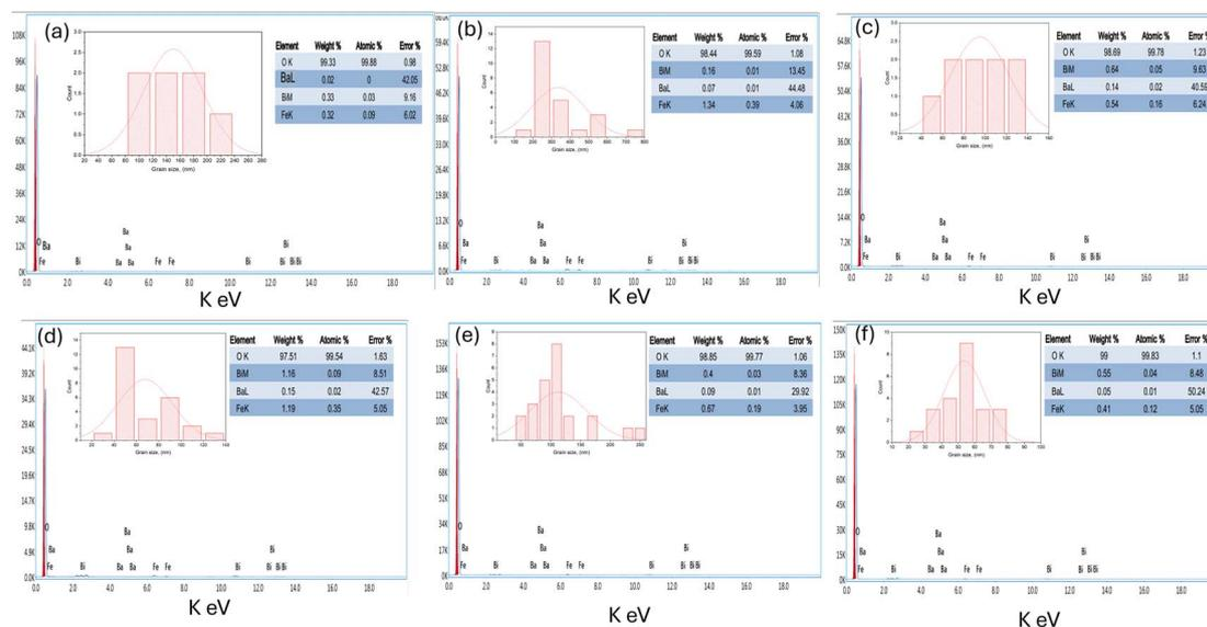
Fig. 6 EDS and percentage of elements, and histogram of particle size of  $\text{Bi}_{0.9}\text{Ba}_{0.1}\text{FeO}_3$  NPs with different fuels: (a) EDTA, (b) glycine, (c) glucose, (d) urea, (e) TEA, and (f) without-fuel.
