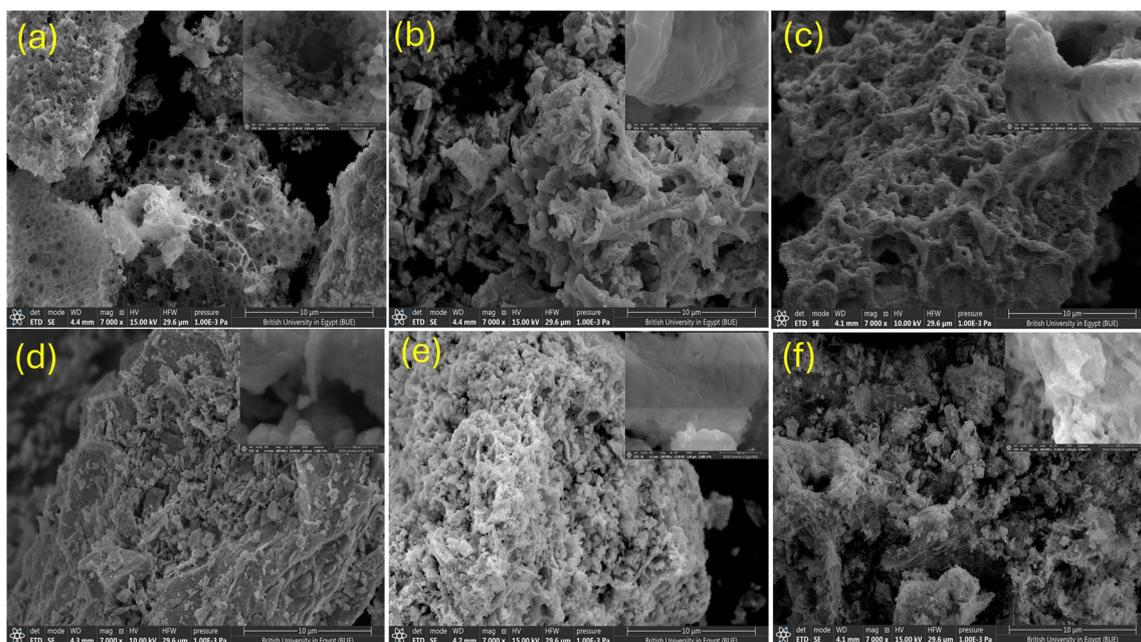
Fig. 5 SEM of  $\text{Bi}_{0.9}\text{Ba}_{0.1}\text{FeO}_3$  at 10 micro-magnifications with different fuels: (a) EDTA, (b) glycine, (c) glucose, (d) urea, (e) TEA, and (f) without-fuel.
