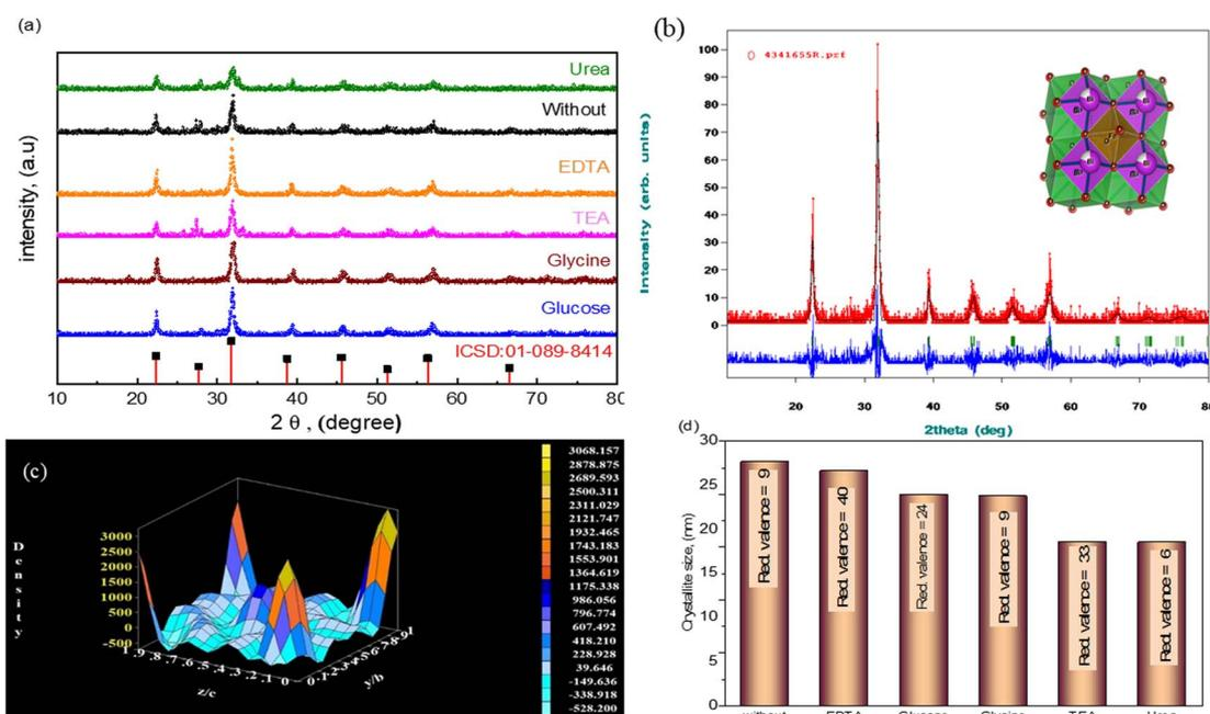
Fig. 3 (a) XRD data of the  $\text{Bi}_{0.9}\text{Ba}_{0.1}\text{FeO}_3$  nanoparticles with different fuels, (b) Rietveld refinement using FullProf software of  $\text{Bi}_{0.9}\text{Ba}_{0.1}\text{FeO}_3$  nanoparticles, (c) X-ray electron density, and (d) crystallite size vs. solvent.
