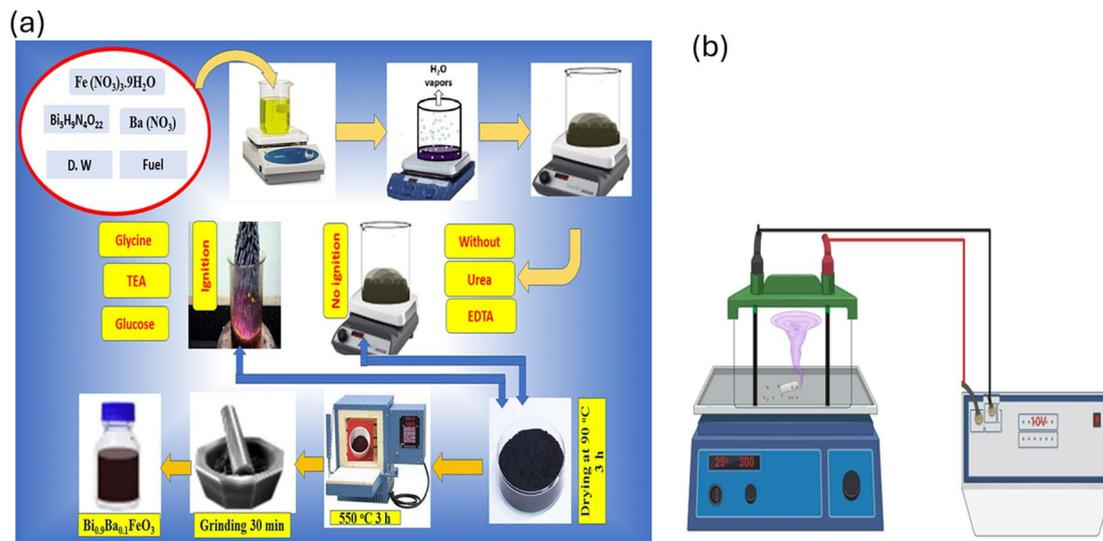
Fig. 2 (a) Scheme of the co-precipitation processes of the nano-Bi<sub>0.9</sub>Ba<sub>0.1</sub>FeO<sub>3</sub> and (b) electrochemical system for degradation of CR dye.
