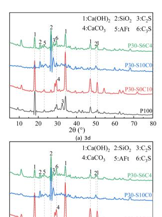
Fig. 5 XRD patterns of samples with different GSGS and GCS ratios. (a) 3 d (b) 28 d
