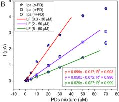
Fig. 8 Electrochemical response of 1-SPGE in the presence of p-PD, o-PD, and m-PD (A) and their calibration curves (B), error bars represent the standard deviation among three replicates (SD, n=3).
