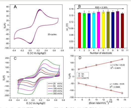
Fig. 5 (A) 20 CV-cycles of modified 1-SPGE at the scan rate of 50 mV s<sup>-1</sup> in 5.0 mM in  $K_3$ [Fe(CN)<sub>6</sub>] solution added with 0.1 M KCl from -0.4 V to 0.7 V potential range. (B) calculated peak to peak potential separation ( $\Delta E_p$ ) of 10 different 1-SPGEs with 3.38% relative standard deviation and y-bar error represents the standard deviation in  $\Delta E_p$  of 20 CV-cycles for each 1-SPGE electrode. (C) and (D) Different scan rates and linear fitting, respectively.
