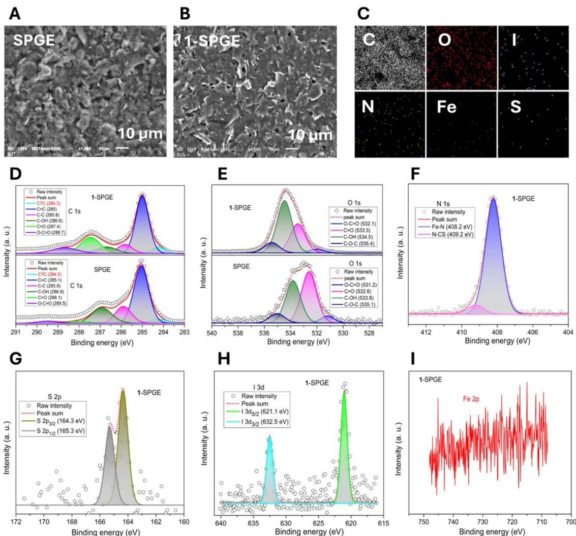
Fig. 4 SEM images of SPGE (A) and 1-SPGE (B); EDX, elemental mapping of 1-SPGE (C); SPGE vs. 1-SPGE XPS spectra comparisons of C 1s (D) and O 1s (E); XPS spectra of other elements in complex **1** of 1-SPGE (F–I) as indicated in the inset of each figure.
