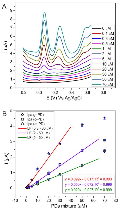
Fig. 8 Electrochemical response of 1-SPGE in the presence of *p*-PD, *o*-PD, and *m*-PD (A) and their calibration curves (B), error bars represent the standard deviation among three replicates (SD,  $n = 3$ ).
