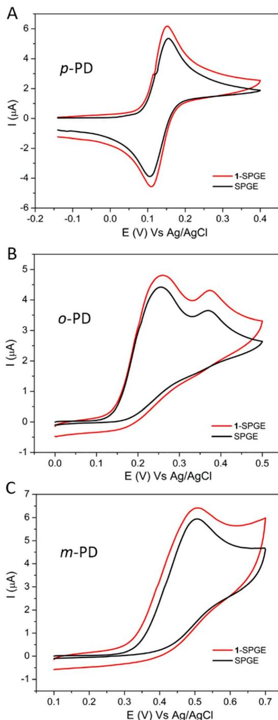
Fig. 6 Cyclic voltammograms of 1-SPGE vs. SPGE added  $100 \mu\text{M}$  concentration of indicated analyte in 0.1 M PBS buffer (pH 7) in aq. 0.1 M KCl at  $50 \text{ mV s}^{-1}$ , (A) *p*-PD (B) *o*-PD and (C) *m*-PD.
