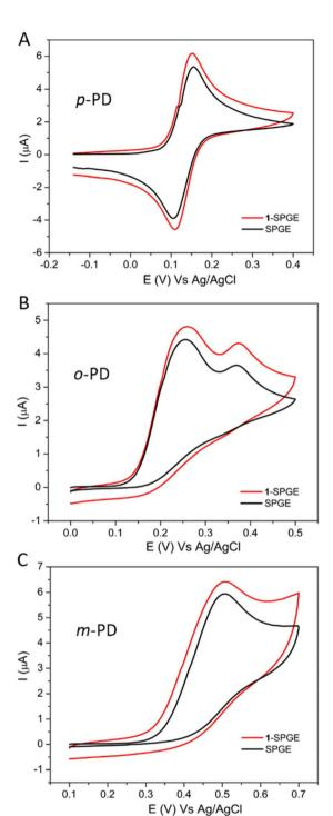
Fig. 6 Cyclic voltammograms of 1-SPGE vs. SPGE added 100  $\mu$ M concentration of indicated analyte in 0.1 M PBS buffer (pH 7) in aq. 0.1 M KCl at 50 mV s<sup>-1</sup>, (A) p-PD (B) o-PD and (C) m-PD.
