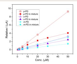
Fig. 9 Comparison of the electrochemical response of 1-SPGE for the separate and simultaneous detection of PD isomers. Error bars are hidden for clarity.
