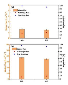
Fig. 7 Separation of binary components. (a) The separation ability of GO membrane for MB/NaCl and RhB/NaCl mixed solutions, (b) separation capacity of GO/CNPs membranes for MB/NaCl and RhB/NaCl mixtures.
