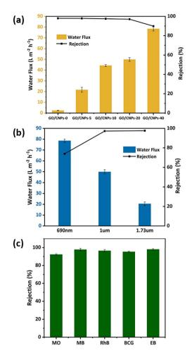
Fig. 5 (a) Water flux and RhB (10 ppm) removal of membranes with CNPs/GO mass ratios of 0, 0.05, 0.1, 0.2, and 0.4, respectively; (b) water flux and RhB (10 ppm) removal of GO/CNPs-20 membranes with different thicknesses; (c) rejection of different dyes (10 ppm) by the GO/CNPs-20 membrane.
