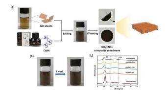
Fig. 1 (a) Schematic diagram of GO/CNPs membrane synthesis process, (b) GO-CNPs mixed solution, (c) XRD of the prepared membranes.
