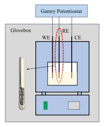
Fig. 1 Three-electrode electrochemical cell setup and pictures of Mg<sup>2+</sup>/Mg reference electrode and alumina container. RE: Mg<sup>2+</sup>/Mg, WE: tungsten or corrosion sample, CE: counter electrode, tungsten.
