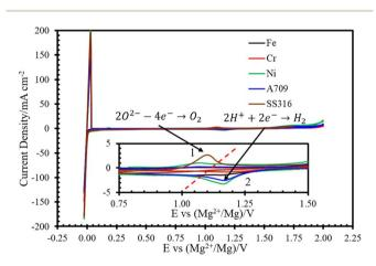
Fig. 2 Cyclic voltammetry scans of each sub-batch salt at 600 °C with scan rate at 100 mV s $^{-1}$ , the WE is tungsten, the RE is Mg $^{2+}$ /Mg, and CE was tungsten.
