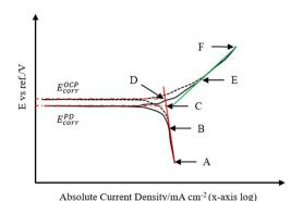
Fig. 6 Theoretical PD curves for illustration of the correlation between the OCP corrosion current density and PD corrosion current density under cathodic diffusion-controlled condition.
