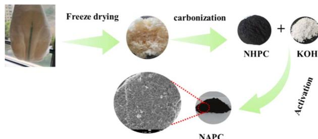
Fig. 1 Schematic of the preparation of porous carbon from diapers.
