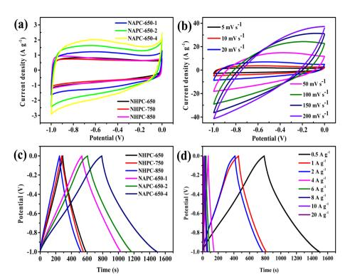
Fig. 7 (a) CV curves of carbon materials in a three-electrode system; (b) CV curves of NAPC-650-4 at different scan rates; (c) constant current charge-discharge curves of carbon materials; (d) CV curves of NAPC-650-4 at various current densities.
