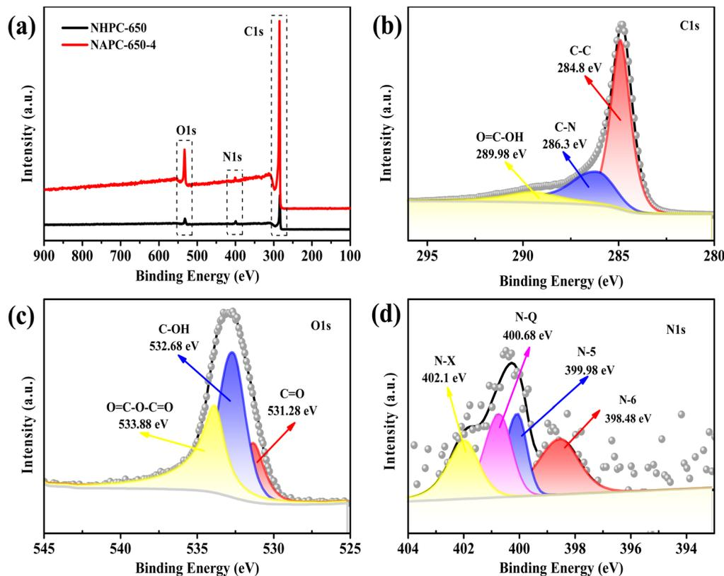
Fig. 6 (a) XPS survey spectrum of NHPC-650 and NAPC-650-4 samples. (b) C 1s peak spectrum of NAPC-650-4 sample. (c) O 1s peak spectrum of NAPC-650-4 sample, and (d) N 1s peak spectrum of NAPC-650-4 sample.
