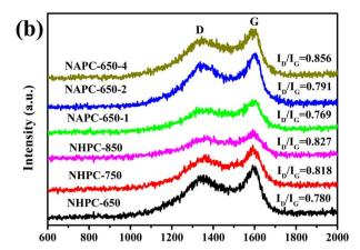
Fig. 4 Carbon materials prepared at different temperatures and KOH activation ratios: (a) XRD patterns and (b) Raman spectra of pyrolytic carbon materials.
