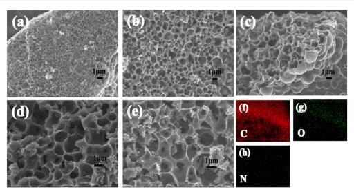
Fig. 2 SEM images: (a) NHPC-650, (b) NAPC-650-1, (c) NAPC-650-2, (d and e) NAPC-650-4, and (f-h) elemental mapping of NAPC-650-4.
