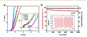
Fig. 8 (a) Nyquist plot of carbon materials in a three-electrode system; (b) charge-discharge test results of NAPC-650-4 at a current density of 10 A g<sup>-1</sup> after 10 000 cycles.
