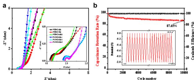
Fig. 8 (a) Nyquist plot of carbon materials in a three-electrode system; (b) charge–discharge test results of NACP-650-4 at a current density of 10  $A g^{-1}$  after 10 000 cycles.
