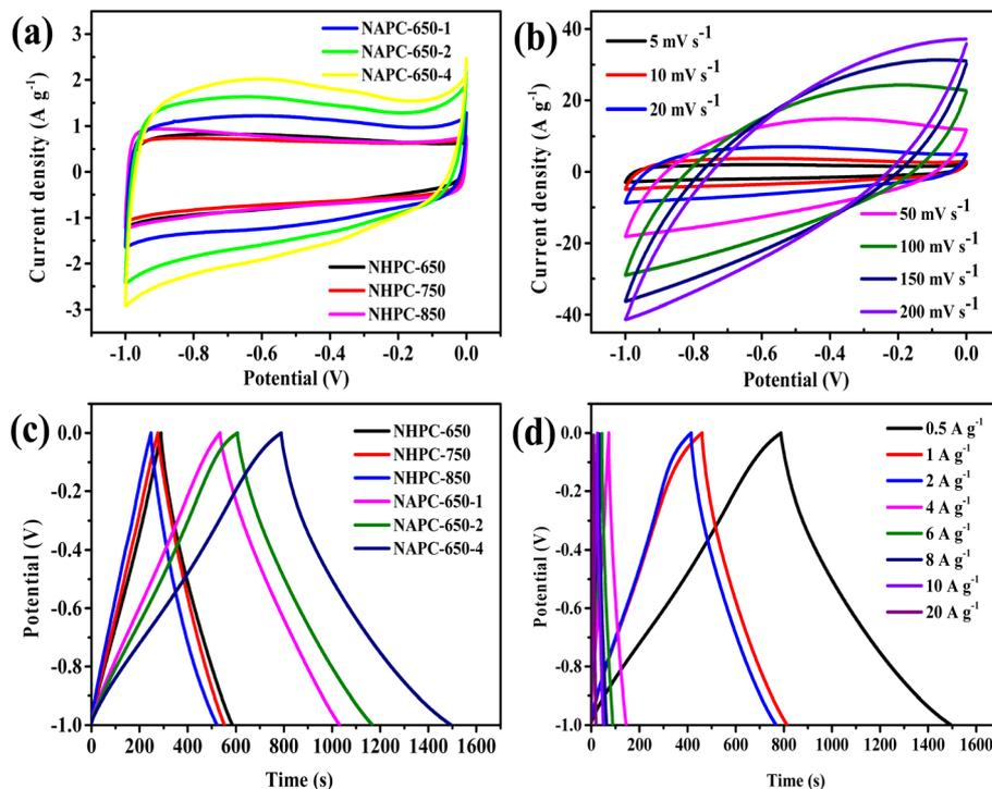
Fig. 7 (a) CV curves of carbon materials in a three-electrode system; (b) CV curves of NACP-650-4 at different scan rates; (c) constant current charge–discharge curves of carbon materials; (d) CV curves of NACP-650-4 at various current densities.
