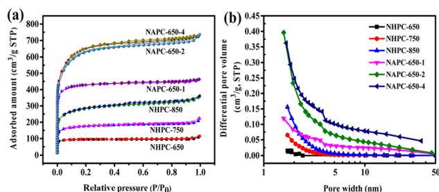
Fig. 3 Carbon materials with various KOH activation ratios: (a) nitrogen adsorption/desorption isotherms and (b) differential pore volume vs. pore width.
