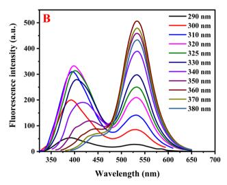
Fig. 3 (A) UV-vis absorption spectra, fluorescence and excitation spectra of NSDC-dots. (B) Fluorescence emission spectra of NSDC-dots after exposing to different excitation wavelengths ranging from 290 to 380 nm.
