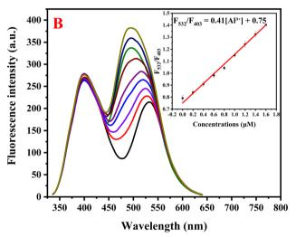
Fig. 4 (A) Fluorescence spectra of NSDC-dots with  ${\rm Co}^{2+}$  concentration range 0–0.7  $\mu$ M. The figure inset shows linear relationship between the fluorescence intensity ratio ( $F_{403}/F_{532}$ ) and the  ${\rm Co}^{2+}$  concentration. (B) Fluorescence spectra of NSDC-dots with Al<sup>3+</sup> concentration range 0–1.6  $\mu$ M. The figure inset shows linear relationship between the fluorescence intensity ratio ( $F_{532}/F_{403}$ ) and the Al<sup>3+</sup> concentration.
