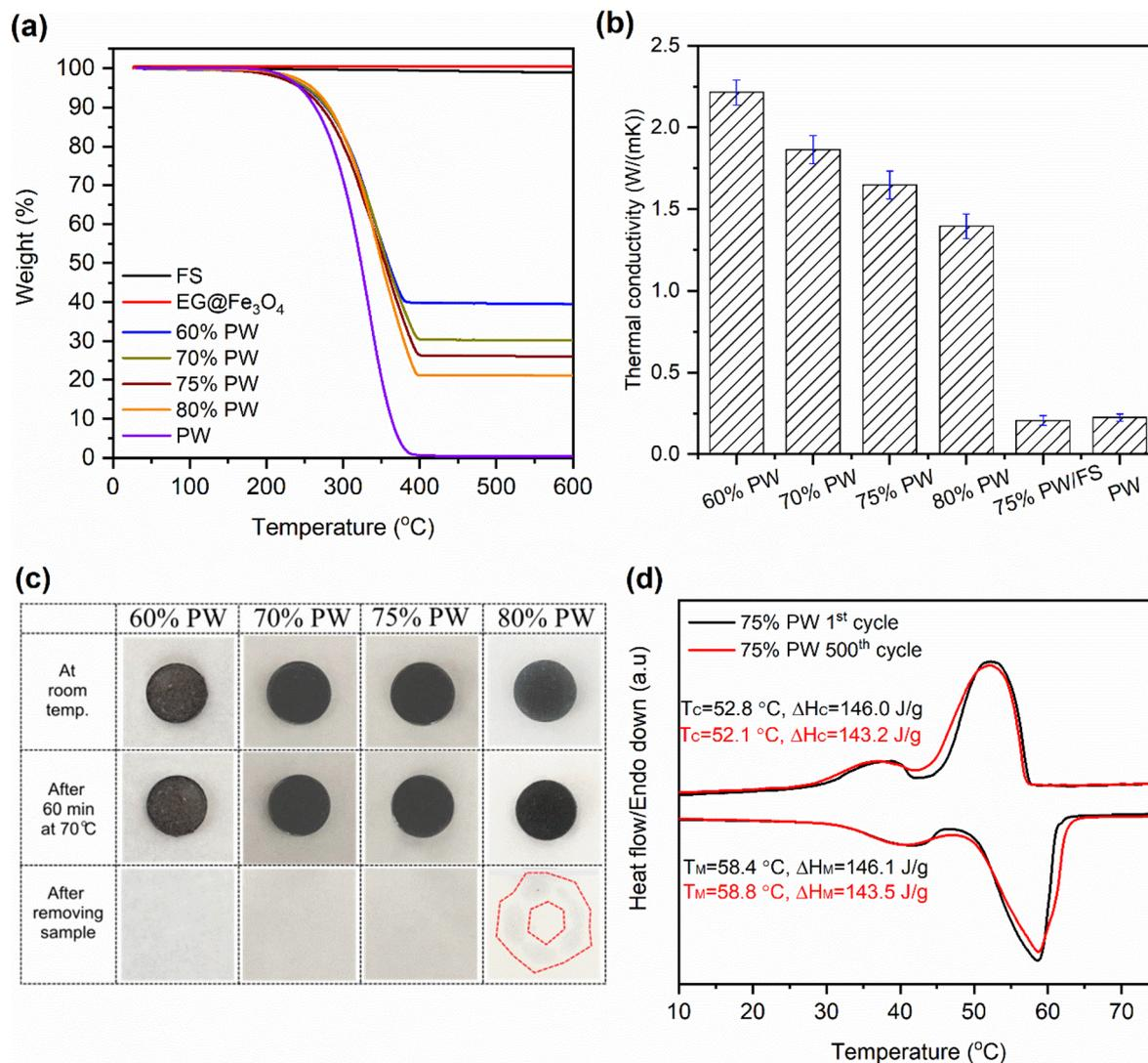
Fig. 6 (a) TGA curves of pristine FS, EG@Fe<sub>3</sub>O<sub>4</sub>, 60–80% PW CPCMs, and pristine PW, and (b) thermal conductivities of 60–80% PW CPCMs and pristine PW, (c) digital photos of 60–80% PW CPCMs during the leakage test, and (d) DSC curves of 75% PW CPCM before and after 500 melting/crystallization cycles.
