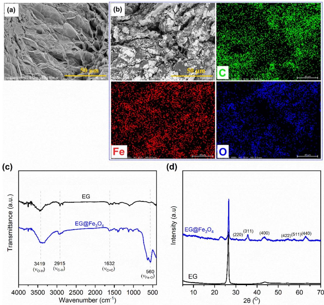
Fig. 1 (a) SEM image of pristine EG, (b) SEM image and corresponding EDS elemental mapping images of EG@Fe<sub>3</sub>O<sub>4</sub>, (c) FTIR spectra of pristine EG and EG@Fe<sub>3</sub>O<sub>4</sub>, and (d) XRD patterns of pristine EG and EG@Fe<sub>3</sub>O<sub>4</sub>.
