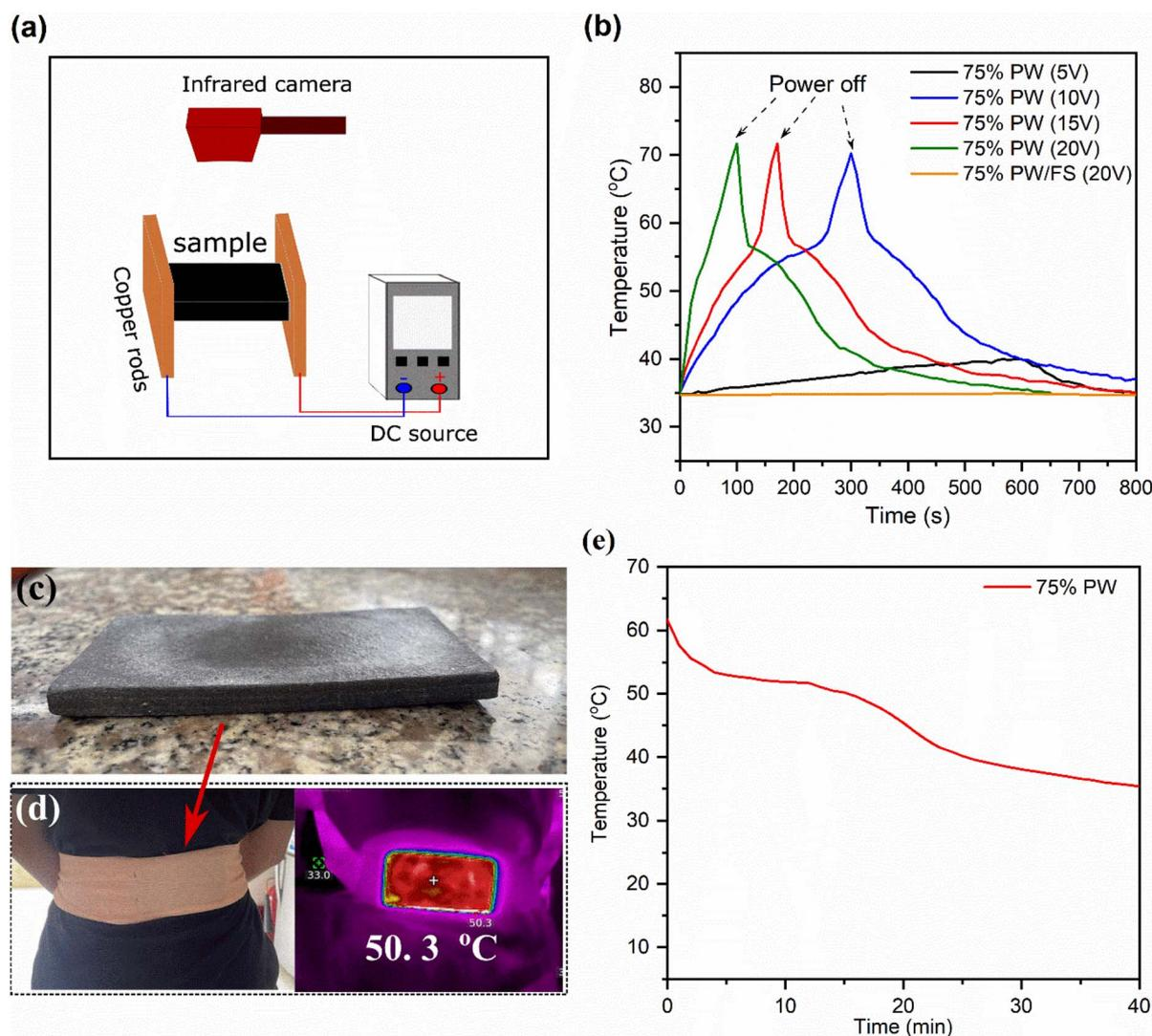
Fig. 8 (a) Illustration of electrothermal conversion apparatus, (b) temperature–time curves of 75% PW/FS/EG@Fe<sub>3</sub>O<sub>4</sub> CPCPM at different applied voltages and 75% PW/FS sample at an applied voltage of 20 V, (c) digital photo of the prepared 75% PW/FS/EG@Fe<sub>3</sub>O<sub>4</sub> heat pack, (d) digital and infrared photos of the 75% heat pack when applied to the back of a volunteer, and (e) temperature–time curve at the center of the pack's inner face during the test.
