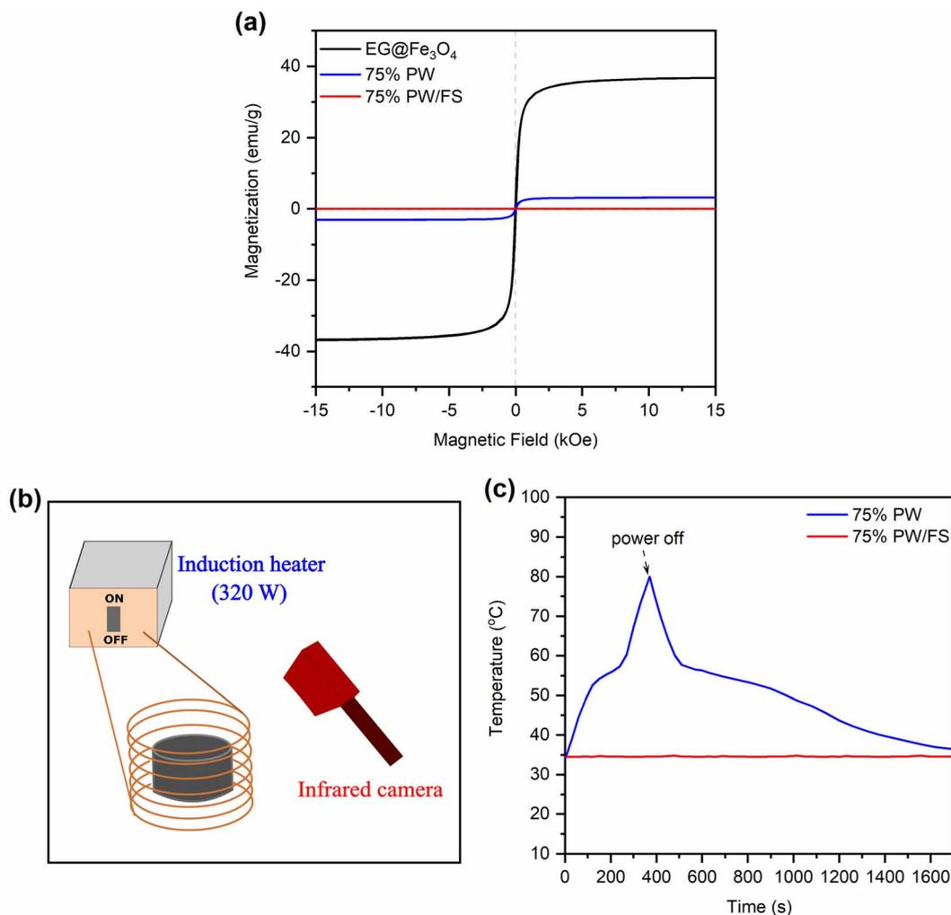
Fig. 7 (a) VSM curves of EG@Fe<sub>3</sub>O<sub>4</sub>, 75% PW/FS/EG@Fe<sub>3</sub>O<sub>4</sub> CPCM, and 75% PW/FS sample, (b) illustration of magnetothermal conversion apparatus, and (c) temperature–time curves of 75% PW/FS/EG@Fe<sub>3</sub>O<sub>4</sub> CPCM and 75% PW/FS sample during magnetothermal conversion and storage experiment.
