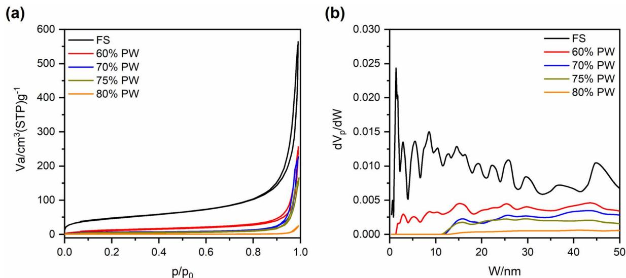
Fig. 3 (a)  $N_2$  adsorption–desorption isotherms and (b) relevant pore size distribution of pristine FS and 60, 70, 75, and 80% PW CPCMs. Note that the data of pristine FS was taken from our previous report.<sup>24</sup>
