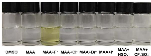
Fig. 3 Visible color changes of MAA observed before and after addition of equal amounts of various tetraethylammonium salts to \text{DMSO} solution ( 1.0 \times 10^{-4} \text{ M} ): from left to right, \text{DMSO} , free MAA , MAA + \text{F}^- , MAA + \text{Cl}^- , MAA + \text{Br}^- , MAA + \text{I}^- , MAA + \text{HSO}_4^- , and MAA + \text{CF}_3\text{SO}_3^- .
