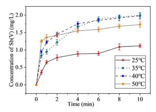
Fig. 4 Effect of reaction temperature on Sb(III) oxidation efficiency. Conditions: reaction temperature: 25 °C, 35 °C, 40 °C, and 50 °C; ozone flow: 0.4 L min<sup>-1</sup>; oxidation time: 10 min; pH: 7; with all other conditions as per Section 2.4.
