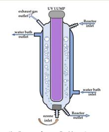
Fig. 1 Schematic diagram of a gas-liquid reactor.
