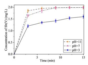
Fig. 6 Effect of different pH values on Sb(III) oxidation efficiency. Conditions: reaction temperature: 35 °C; ozone flow: 0.3 L min<sup>-1</sup>; pH: 3, 7, and 11; with all other conditions as per Section 2.4.
