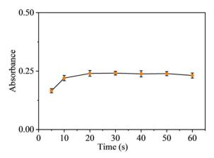
Fig. 11 Effect of sonication time on LLME. Conditions: hydrochloric acid concentration in the 10 mL sample:  $2.4 \text{ mol L}^{-1}$ ; with all other steps as per Section 2.4.
