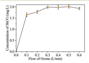
Fig. 5 Effect of ozone flow on Sb(iii) oxidation efficiency. Conditions: reaction temperature: 35 °C; ozone flow: 0.1 L min $^{-1}$ , 0.2 L min $^{-1}$ , 0.3 L min $^{-1}$ , 0.4 L min $^{-1}$ , 0.5 L min $^{-1}$ , and 0.6 L min $^{-1}$ ; oxidation time: 10 min; pH: 7; with all other conditions as per Section 2.4.
