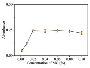
Fig. 10 Effect of malachite green concentration on LLME. Conditions: hydrochloric acid concentration in the 10 mL sample:  $2.4 \text{ mol L}^{-1}$ ; with all other steps as per Section 2.4.
