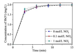
Fig. 8 Effect of  $NO^{3-}$  concentration on Sb(iii) oxidation efficiency. Conditions:  $NO_3^-$  concentration:  $0.1 \, \text{mol L}^{-1}$  and  $1 \, \text{mol L}^{-1}$ ; pH: 7; with all other steps as per Section 2.4.
