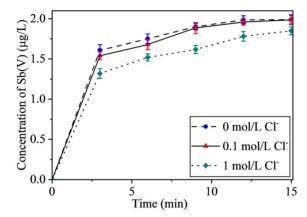
Fig. 7 Effect of  $Cl^-$  concentration on Sb(III) oxidation efficiency. Conditions:  $Cl^-$  concentration: 0.1 mol  $L^{-1}$  and 1 mol  $L^{-1}$ ; pH: 5–6, with all other conditions as per Section 2.4.
