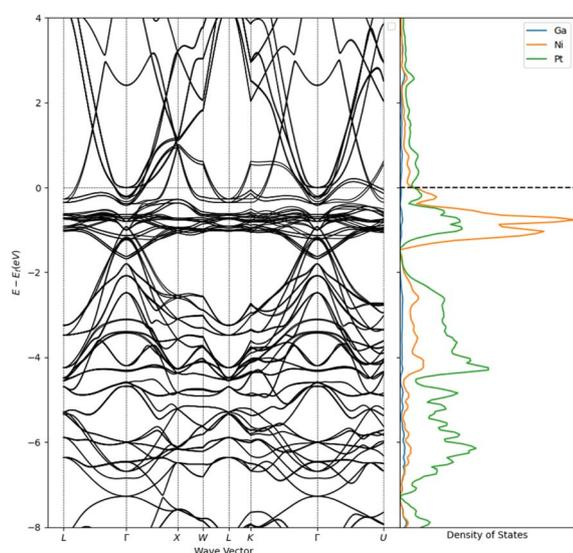
Fig. 3 DFT computed band structure of  $\text{NiPt}_2\text{Ga}$  in the tetragonal Heusler structure with lattice parameters determined from experimental data along high symmetry directions. DOS computed for total Ga, Ni, and Pt contributions.
