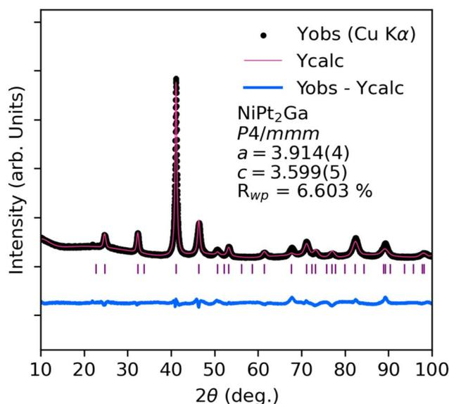
**Fig. 2** Powder X-ray diffraction of phase pure NiPt<sub>2</sub>Ga Rietveld refinement using the  $P4/mmm$  tetragonal Heusler structure.
