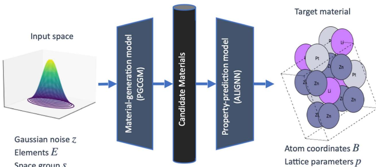
Fig. 1 The PGCGM is a GAN that maps a sample of random Gaussian noise  $z$ , three elements  $E$ , and a space group  $s$  to a ternary unit cell structure as characterized by its atom coordinates  $B$  and lattice parameters  $p$ . Varying  $z$  enables different structures with the same elements and space group to be generated. We generate 27 116 structures with the PGCGM and then use a GNN to predict the decomposition enthalpy of each structure.
