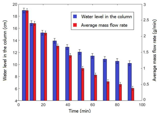
Fig. 3 Correlation between the water level in the column and the average mass flow rate through the nanocomposite ceramic.
