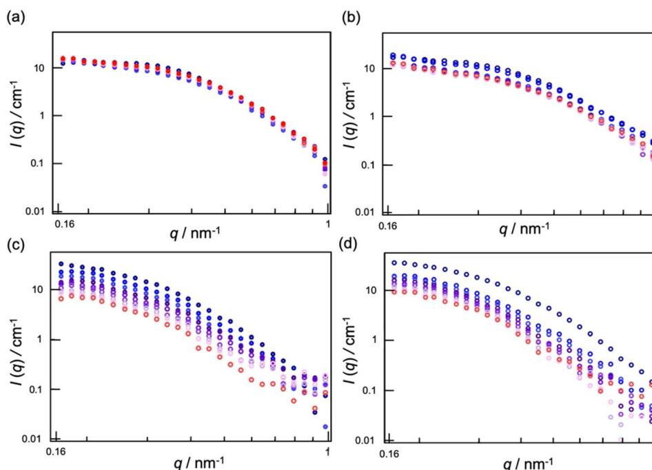
Fig. 4 SANS profiles of (a) 1/6 d-ME applied to dry SC, (b) 1/9 d-ME applied to dry SC, (c) 1/6 d-ME applied to hydrated SC, and (d) 1/9 d-ME applied to hydrated SC. The color changed over time from blue to red.
