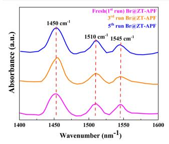
Fig. 9 Pyridine IR spectra of Br@ZT-APF catalyst after evacuation at 150  $^{\circ}\text{C}.$
