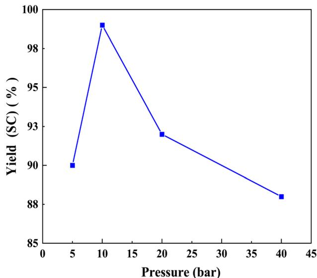
Fig. 7 Effect of CO<sub>2</sub> pressure on SC yield over Br@ZT-APF. Reaction conditions: catalyst mass = 200 mg temperature = 120 °C: reaction time = 4 h: amount of styrene oxide = 3.5 mL: amount ACN (10 mL) as solvent.
