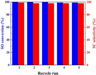
Fig. 8 Catalyst recyclability study for cycloaddition reaction over Br@ZT-APF. Reaction conditions; catalyst mass = 200 mg;  $CO_2$  pressure = 10 bar; temperature = 120 °C; reaction time = 4 h; amount of styrene = 3.5 mL; amount ACN (10 mL) as solvent.
