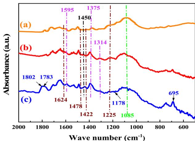
Fig. 10 The FTIR spectra of the Br@ZT-APF. (a) Before reaction, (b) after reaction, (c) adsorption of catalyst with CO<sub>2</sub>.
