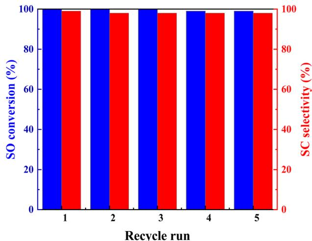
Fig. 8 Catalyst recyclability study for cycloaddition reaction over Br@ZT-APF. Reaction conditions; catalyst mass = 200 mg; CO<sub>2</sub> pressure = 10 bar; temperature = 120 °C; reaction time = 4 h; amount of styrene = 3.5 mL; amount ACN (10 mL) as solvent.
