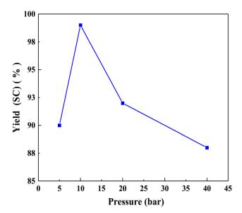
Fig. 7 Effect of  $CO_2$  pressure on SC yield over Br@ZT-APF. Reaction conditions: catalyst mass = 200 mg temperature = 120 °C: reaction time = 4 h: amount of styrene oxide = 3.5 mL: amount ACN (10 mL) as solvent.
