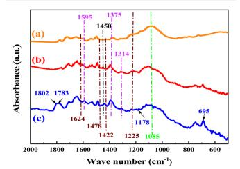
Fig. 10 The FTIR spectra of the Br@ZT-APF. (a) Before reaction, (b) after reaction, (c) adsorption of catalyst with CO2.
