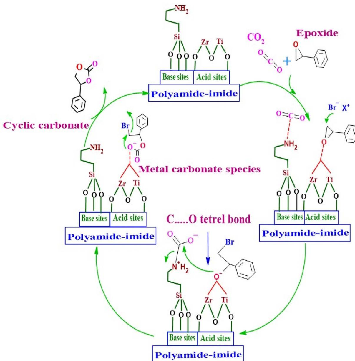
Scheme 2 The proposed reaction mechanism for cycloaddition of epoxide and CO<sub>2</sub>, as catalyzed by Br@ZT-APF.
