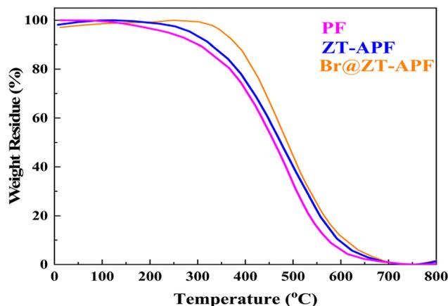
Fig. 5 TGA plots for catalysts.
