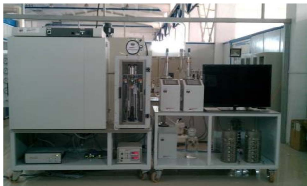
Fig. 2 Minimum miscible pressure measurement instrument.
