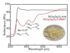
Fig. 5 UV-vis diffuse reflectance spectra of  $SrCa_2Ga_2O_6$  (black) and  $SrCa_2Ga_2O_6$ :0.03Mn<sup>4+</sup> (red). The insert photograph is the body color of  $SrCa_2Ga_2O_6$ :0.03Mn<sup>4+</sup> under fluorescent light.
