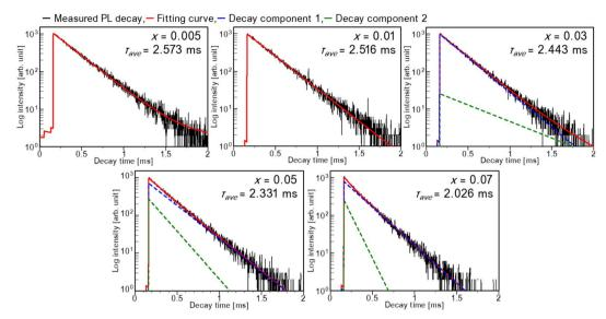
Fig. 7 PL decay curves of  $SrCa_2Ga_2O_6$ : $xMn^{4+}$  (0.005  $\leq x \leq$  0.07) monitored at 712 nm excited at 365 nm.
