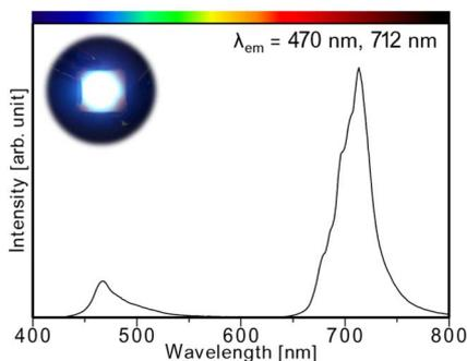
Fig. 10 Luminescence spectra of 470 nm blue LED chip packaged with SrCa<sub>2</sub>Ga<sub>2</sub>O<sub>6</sub>:0.03Mn<sup>4+</sup> powder under 10 mA current. The insert photograph is the prepared LED device emitting blue and deep-red light.
