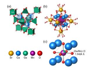
Fig. 3 (a) The tetrahedral cluster constructed by  $[Ga2O_4]$ ,  $[Ca2O_5]$ ,  $[Ga3O_4]$ , and  $[Ga4O_8]$  centered on O2. (b) The octahedral cluster formed by  $[Sr1O_9]$  and  $[Ca1O_6]$  centered on  $[(Ga1/Mn1)O_6]$  octahedron. (c) The aristotype perovskite-like structure composed of Ga1/Mn1, Ca1, and O1.
