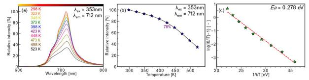
Fig. 9 (a) Temperature-dependent PL spectra of  $SrCa_2Ga_2O_6$ :0.03Mn<sup>4+</sup>. (b) The plot of relative emission intensities at each temperature. (c) Arrhenius plot of relative emission intensities for  $SrCa_2Ga_2O_6$ :0.03Mn<sup>4+</sup>.
