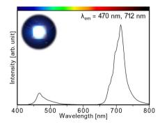
Fig. 10 Luminescence spectra of 470 nm blue LED chip packaged with  $SrCa_2Ga_2O_6$ :0.03Mn<sup>4+</sup> powder under 10 mA current. The insert photograph is the prepared LED device emitting blue and deep-red light.
