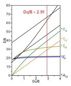
Fig. 8 Tanabe—Sugano energy level diagram of Mn<sup>4+</sup> at octahedrally coordinated environment. Red line indicates the crystal filed strength of Mn<sup>4+</sup> in the SrCa<sub>2</sub>Ga<sub>2</sub>O<sub>6</sub> host lattice.
