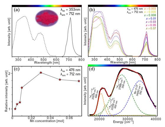
Fig. 6 (a) PL and PLE spectra of  $SrCa_2Ga_2O_6$ :  $0.03Mn^{4+}$ . The insert photograph is emission color of  $SrCa_2Ga_2O_6$ :  $0.03Mn^{4+}$  under 365 nm n-UV irradiation. (b) PL and PLE spectra of  $SrCa_2Ga_2O_6$ :  $Xmn^{4+}$  ( $0 \le x \le 0.07$ ) excited at 476 nm. (c) Dependence of emission intensities of  $SrCa_2Ga_2O_6$ :  $SrCa_2Ga$
