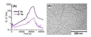
Fig. 2 (A) Rheological time-sweeps of G' and G'' (0.5% strain, 1 Hz at 20 °C) of 1 mM aqueous gels of  $K_21a$  prepared with 0.05 M glucono- $\delta$ -lactone (GdL). (B) Cryo-TEM image of the hydrogel formed with  $K_21a$  (c=1.0 mM) and glucono- $\delta$ -lactone (GdL) 0.05 M.
