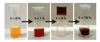
Fig. 1 Gelation of 1 mM K<sub>2</sub>1a using 0.05 M glucono-δ-lactone (GdL).
