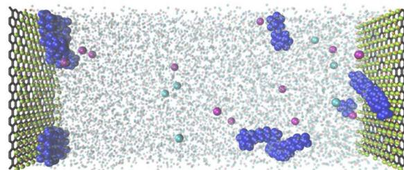
Fig. 5 Snapshot of an MD simulation. Molecules are colored as  $C_{16}$ TAB: blue, sodium ion: aqua, bromide ion: purple, hydroxyl groups: pink and yellow. Water molecules are illustrated transparently. The slab size is  $24.595 \text{ \AA} \times 42.6 \text{ \AA} \times 100.64 \text{ \AA}$ , where the graphene is configured with 10 hexagonal lattices. The numbers of molecules are water: 3094,  $C_{16}$ TAB: 6, and NaBr: 6.
