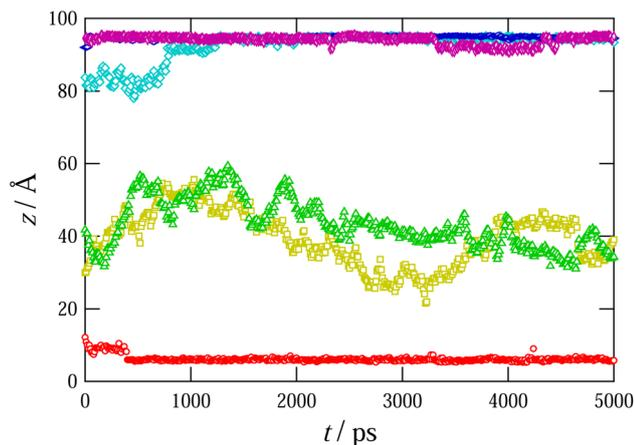
Fig. 6 Time evolution of the positions of the N molecules in the surfactant molecules in the direction perpendicular to the GO membranes ( $z$ -direction). Different symbols are used to distinguish different molecules. The GO membranes are located at  $z = 0, 100.64 \text{ \AA}$ .
