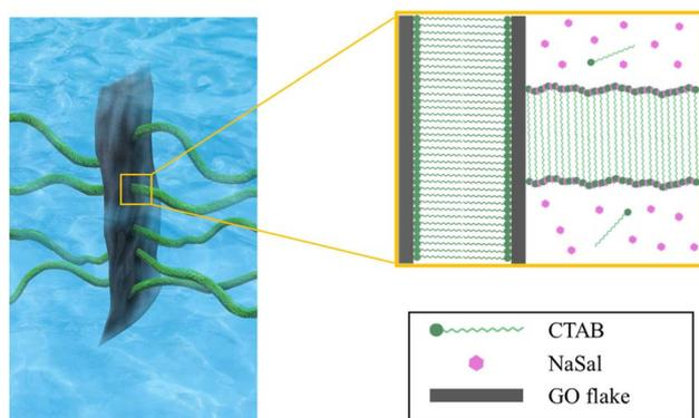
Fig. 8 Schematic of the micellar structure in a GO/C<sub>16</sub>TAB/NaSal dispersion.
