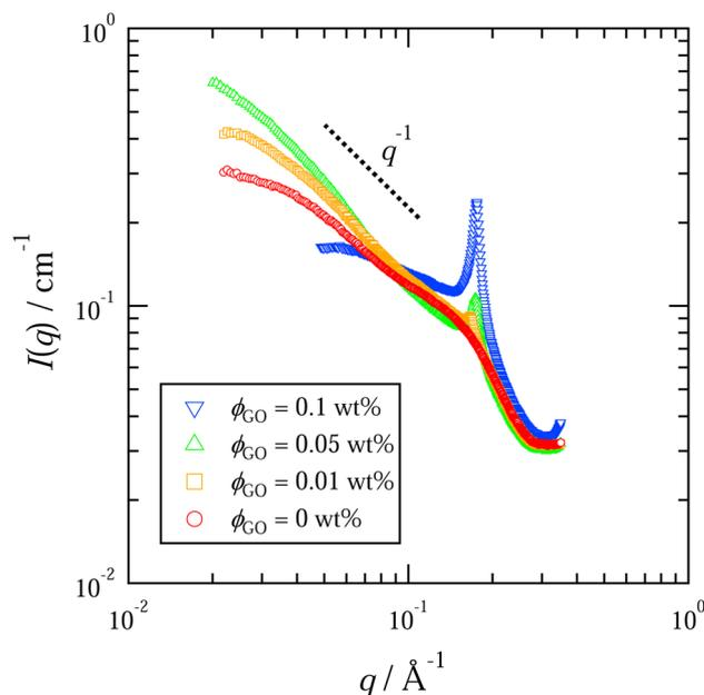
Fig. 3 Scattering intensity  $I(q)$  as a function of the magnitude of the scattering vector  $q$ . Results for the system with  $C_{\text{D}} = 100$  mM are shown. Different symbols represent different concentrations of GO,  $\phi_{\text{GO}}$ . The dashed line depicts the inverse proportional scaling relation  $I(q) \sim q^{-1}$  that is typical behavior for rod-like particles.
