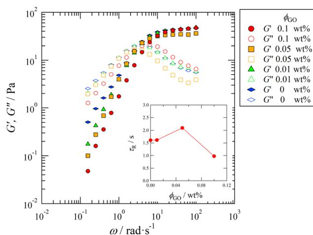
Fig. 2 Log–log plot of the elastic modulus  $G'$  and loss modulus  $G''$  as a function of the frequency  $\omega$  at  $C_{\text{D}} = 100$  mM. Symbols distinguish the concentration of the GO,  $\phi_{\text{GO}}$ , as indicated in the legend. (Inset) The stress relaxation time  $\tau_{\text{R}} = 2\pi/\omega_{\text{CO}}$  as a function of  $\phi_{\text{GO}}$ . The crossover frequency  $\omega_{\text{CO}}$  is estimated by fitting the results to the single Maxwell model.
