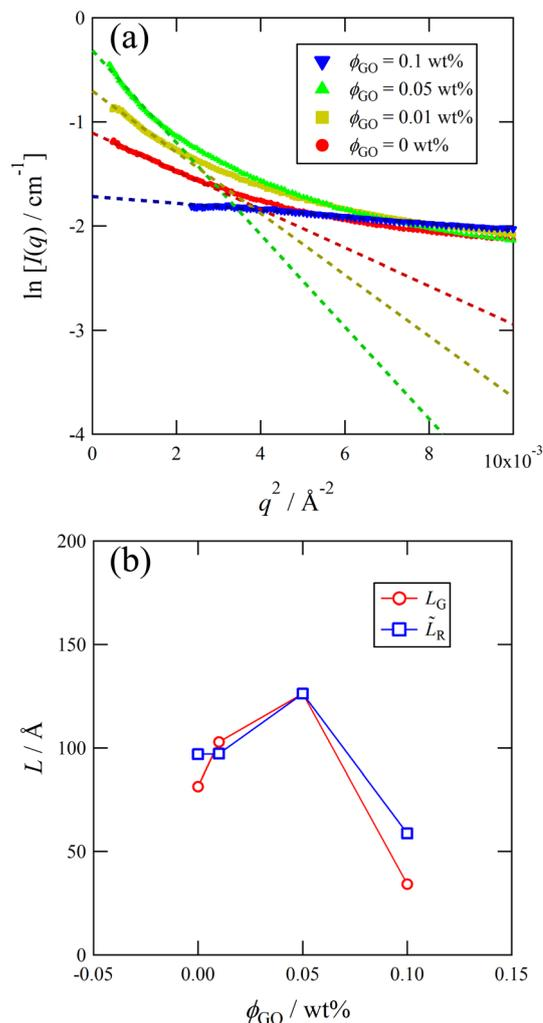
Fig. 7 (a) Guinier plot of SAXS profiles with varying  $\phi_{GO}$ . The dashed line represents the fitted line of the Guinier model. (b)  $\phi_{GO}$  dependence of  $L_G$  estimated from Guinier plot and  $\tilde{L}_R = L_R \times (L_G^{\max}/L_R^{\max})$  estimated from viscoelastic measurements.
