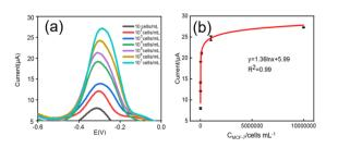
Fig. 6 (a) Current response of the biosensor to the different concentration of MCF-7 cancer cells. (b) The relationship of the current response and cancer cells concentration.
