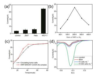
Fig. 5 Current response of biosensor. (a) Current response of chip to different kinds of cells. (b) Effect of the coupling ratio of HRP to  $Ab_2$  on the electrochemical performance of the biosensor. (c) Effect of incubation time of cancer cells and HRP-MWCNT-COOH- $Ab_2$  complex on the electrochemical performance of the biosensor. (d) Current response of the chip under different condition.
