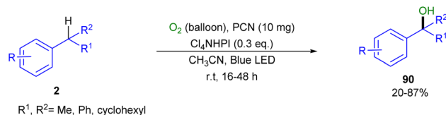
Scheme 56 Photocatalytic hydroxylation of benzylic C(sp 3 )-H bonds using O 2 (Das and co-workers). 54
