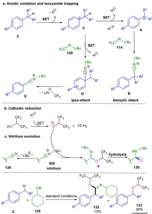
Scheme 82 Possible mechanism for the electrochemical carbamoylation and cyanation of benzylic C(sp<sup>3</sup>)-H bonds.
