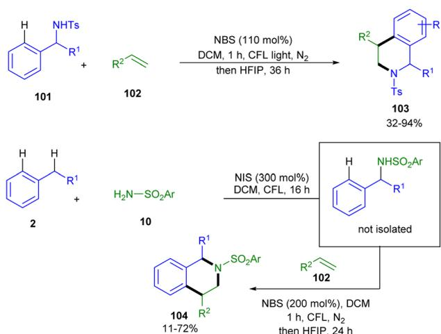
Scheme 63 Reaction of toluene derivatives with sulfonamides and olefins (Li and co-workers).<sup>59</sup>
