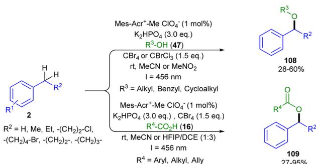
Scheme 66 Benzylic C(sp<sup>3</sup>)-H etherification and esterification reactions via photoredox catalysis (Das and co-workers).<sup>61</sup>
