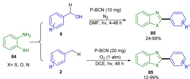
Scheme 50 P-BCN-catalyzed alcohol oxidation/toluene C(sp<sup>3</sup>)-H activation with *o*-thio/hydroxy/aminoanilines (Jiang and co-workers).<sup>51</sup>
