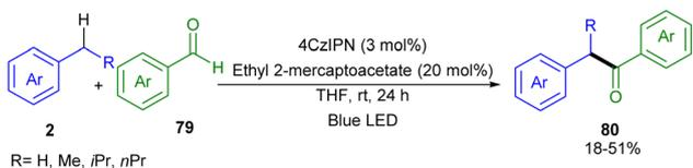
Scheme 46 Photocatalytic cross-coupling of the benzylic C–H bond of toluene with aromatic aldehydes (Guo and co-workers).<sup>49</sup>
