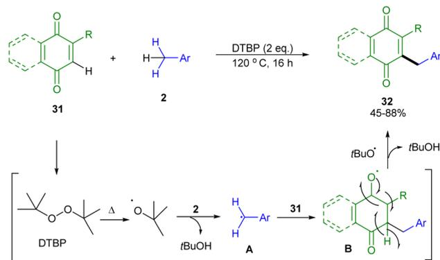
Scheme 18 DTBP-mediated cross-coupling of quinones with benzylic C(sp<sup>3</sup>)-H bonds (Wang and co-workers).<sup>30</sup>
