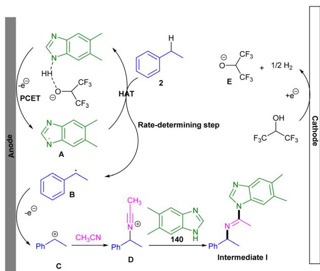
Scheme 89 Plausible mechanism for benzylic C(sp<sup>3</sup>)-H amination in the presence of benzimidazole and acetonitrile.
