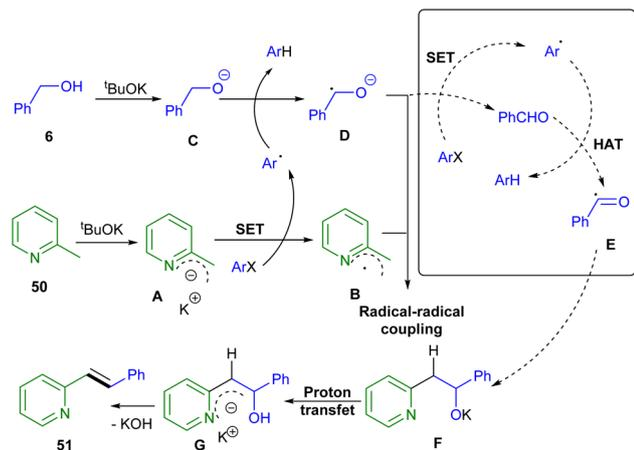
Scheme 28 Possible mechanism for the KOtBu-promoted C(sp<sup>3</sup>)-C(sp<sup>3</sup>) cross-coupling between methyl N-heteroarenes and benzylic alcohols.
