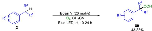
Scheme 54 Benzylic C(sp<sup>3</sup>)-H activation/hydroperoxidation using O<sub>2</sub> (Xing and co-workers).<sup>55</sup>
