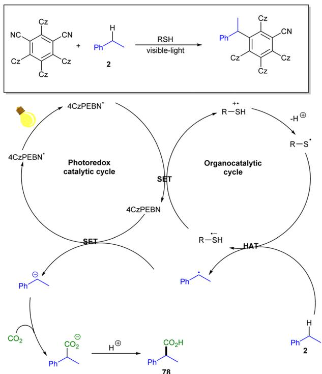
Scheme 45 Catalytic cycle for the photocarboxylation of benzylic C–H bonds using CO<sub>2</sub>.
