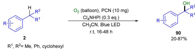
Scheme 56 Photocatalytic hydroxylation of benzylic C(sp<sup>3</sup>)-H bonds using O<sub>2</sub> (Das and co-workers).<sup>54</sup>
