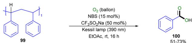
Scheme 62 Upcycling of polystyrene-based wastes into low weight aromatics (Das and co-workers).<sup>58</sup>
