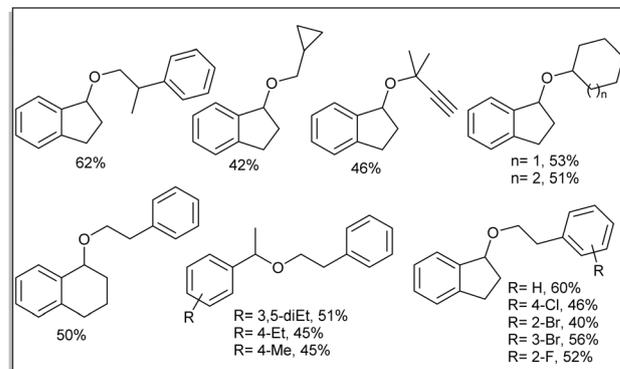
Scheme 87 Electrochemical etherification of benzylic C-H bonds with alcohols (Wang and co-workers).<sup>75</sup>
