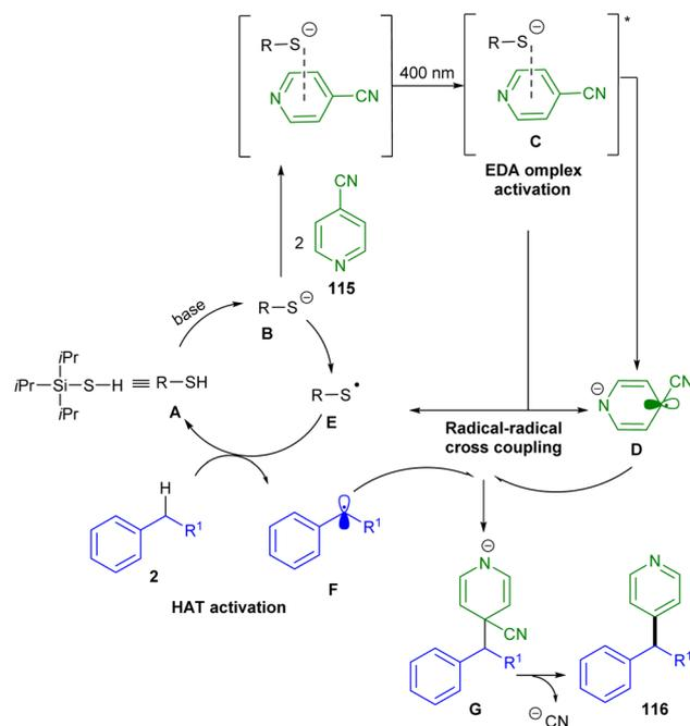
Scheme 72 Reasonable mechanism for visible light-induced redox-neutral heteroarylation of C(sp<sup>3</sup>)-H bonds.
