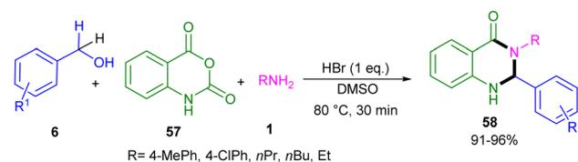
Scheme 31 Oxidative C(sp<sup>3</sup>)-N coupling using HBr and DMSO towards 2,3-dihydroquinazolin-4(1*H*)-ones (Rashidi Ranjbar and co-workers).<sup>40</sup>
