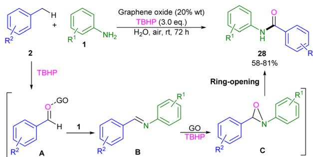
Scheme 15 Graphene oxide/TBHP-catalyzed reaction of toluene with aniline (Dandia and co-workers).<sup>28</sup>
