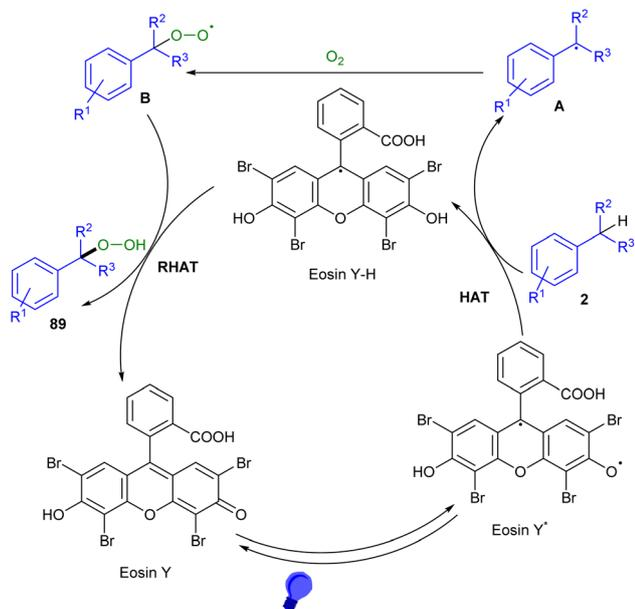
Scheme 55 Photocatalytic cycle for C(sp<sup>3</sup>)-H activation/hydroperoxidation using O<sub>2</sub>.
