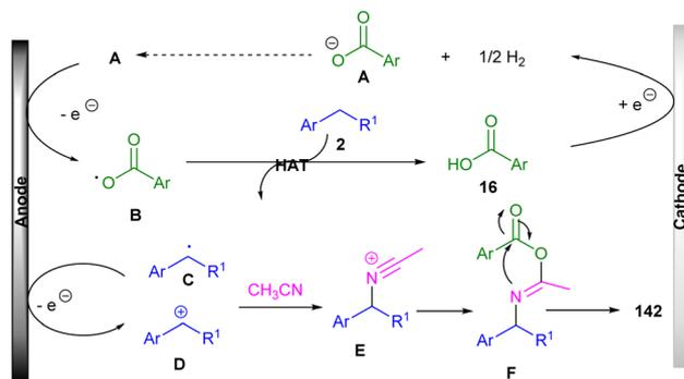
Scheme 91 Rational mechanism for electrochemical benzylic C(sp<sup>3</sup>)-H amidation using benzoic acid and acetonitrile.
