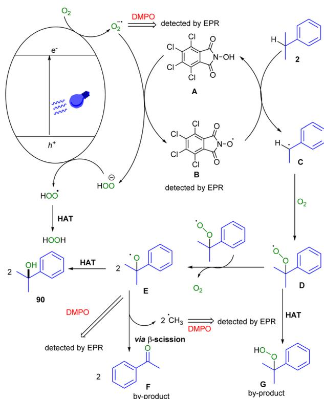
Scheme 57 Catalytic cycle for the photocatalytic hydroxylation of benzylic C(sp<sup>3</sup>)-H bonds using O<sub>2</sub>.
