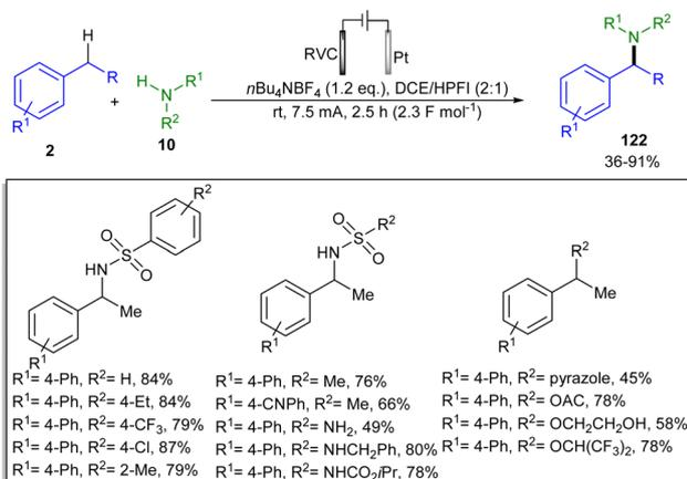
Scheme 76 Electrochemical C–H amination of toluene with amine and oxygen nucleophiles (Xu and co-workers).<sup>68</sup>
