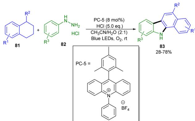
Scheme 48 C(sp<sup>3</sup>)-H activation/annulation of tetrahydronaphthalenes (Shen and co-workers).<sup>50</sup>
