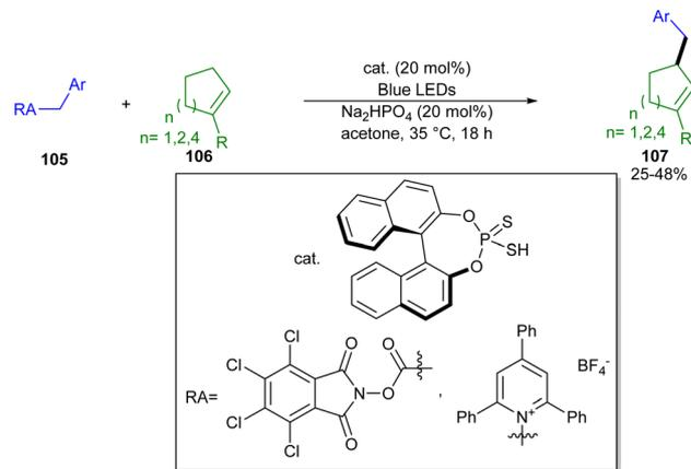
Scheme 64 Photoredox catalytic allylation of benzylic C(sp<sup>3</sup>)-H bonds (Melchiorre and co-workers).<sup>60</sup>
