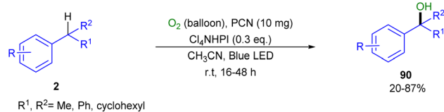
Scheme 56 Photocatalytic hydroxylation of benzylic C(sp 3 )-H bonds using O 2 (Das and co-workers). 54
