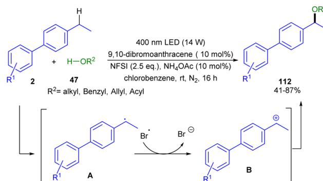
Scheme 69 Visible light-driven organocatalytic alkoxylation of benzylic C-H bonds (Dai and co-workers).<sup>63</sup>
