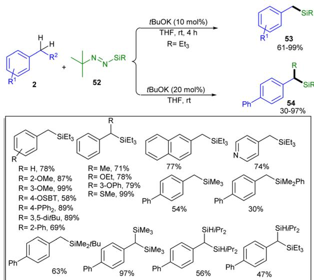
Scheme 29 KOtBu-catalyzed silylation of benzylic C(sp<sup>3</sup>)-H bonds (Chauvier and co-workers).<sup>38</sup>
