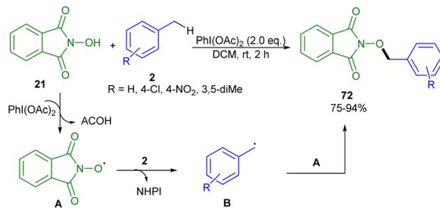
Scheme 39 Iodine(III)-promoted coupling of *N*-hydroxyphthalimide (NHPI) with unactivated C(sp<sup>3</sup>)-H bonds (Wu and co-workers).<sup>45</sup>
