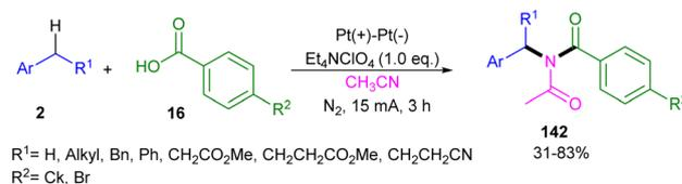
Scheme 90 Electrochemical benzylic C(sp<sup>3</sup>)-H amidation using benzoic acid and acetonitrile (Qian and co-workers).<sup>77</sup>
