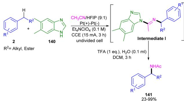
Scheme 88 Benzylic C(sp<sup>3</sup>)-H amination in the presence of benzimidazole and acetonitrile (Zhang and co-workers).<sup>76</sup>
