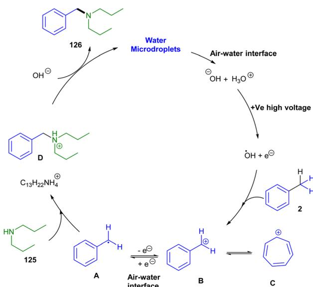
Scheme 79 Rational mechanism for the C(sp<sup>3</sup>)-H amination of toluene with amine in the presence of water microdroplets.
