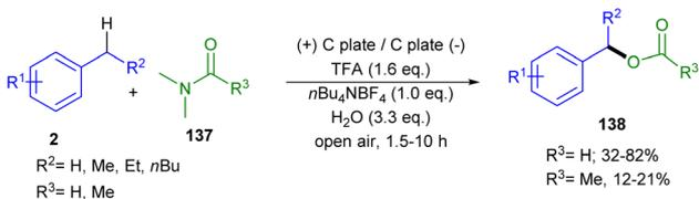
Scheme 85 Electrochemical formyloxylation of benzylic  $C(sp^3)$ -H bonds with DMF (Guan and co-workers).<sup>74</sup>
