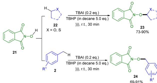
Scheme 11 Synthesis of *N*-alkoxyphthalimides through ultrasound acceleration (Gui and co-workers).<sup>26</sup>
