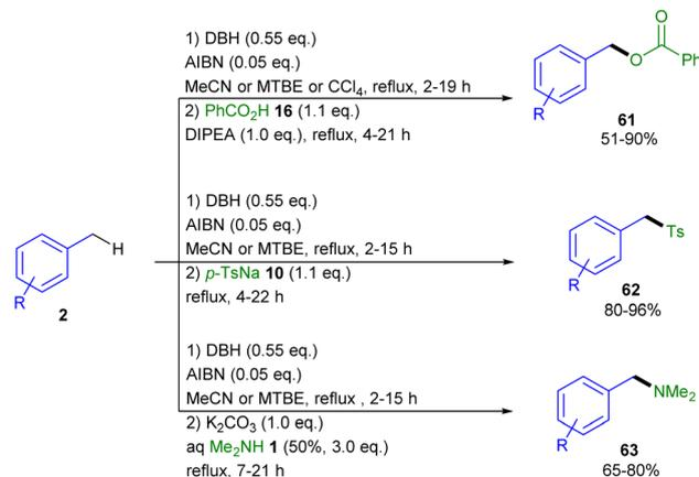
Scheme 34 Metal-free formation of C–O, C–S, and C–N bonds at the benzylic position of toluene (Togo and co-workers).<sup>42</sup>
