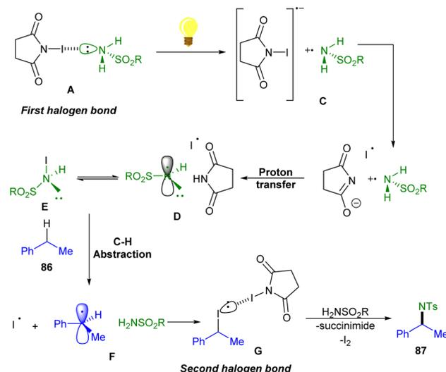
Scheme 53 Possible mechanism for the C(sp<sup>3</sup>)-H activation/amination of arylalkyl substrates.
