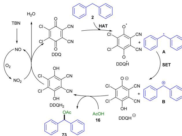
Scheme 41 Possible mechanism for aerobic oxidative C-O coupling of C(sp<sup>3</sup>)-H with carboxylic acids.
