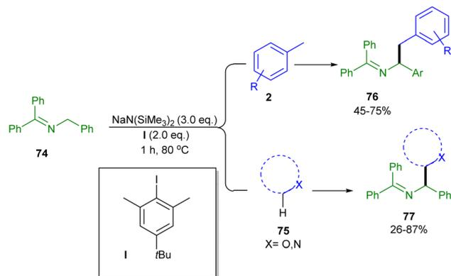
Scheme 42 C(sp<sup>3</sup>)-H/C(sp<sup>3</sup>)-H dehydrogenative coupling of saturated heterocycles and toluene with *N*-benzyl imines (Zhang and co-workers).<sup>47</sup>
