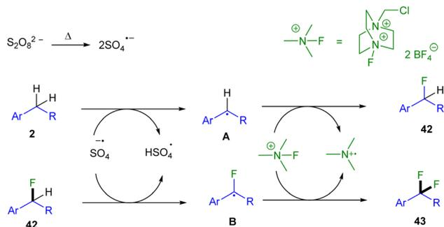
Scheme 23 Proposed mechanism for K<sub>2</sub>S<sub>2</sub>O<sub>8</sub>-promoted selective benzylic mono- and di-fluorination.
