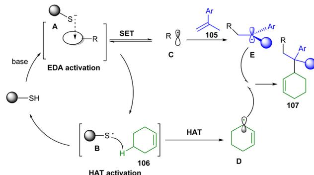
Scheme 65 Rational mechanism for photoredox catalytic allylation of benzylic C(sp<sup>3</sup>)-H bonds.
