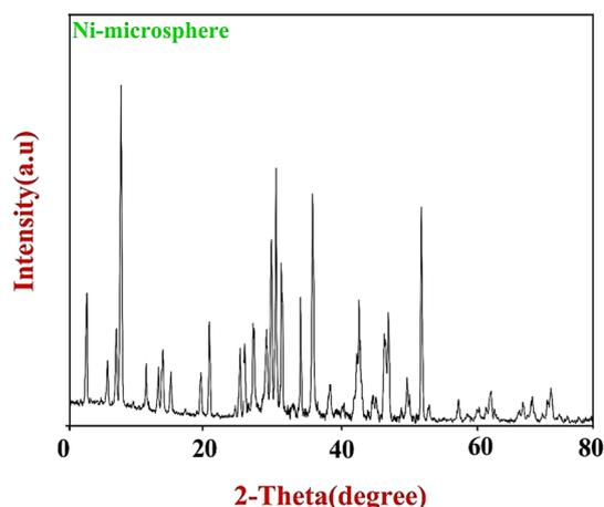
Fig. 2 XRD pattern of Ni-ascorbic acid MOF.
