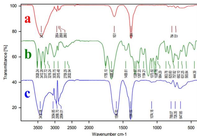
Fig. 1 FT-IR spectra of (a) Ni(NO<sub>3</sub>)<sub>2</sub>, (b) ascorbic acid, and (c) Ni-ascorbic acid MOF.
