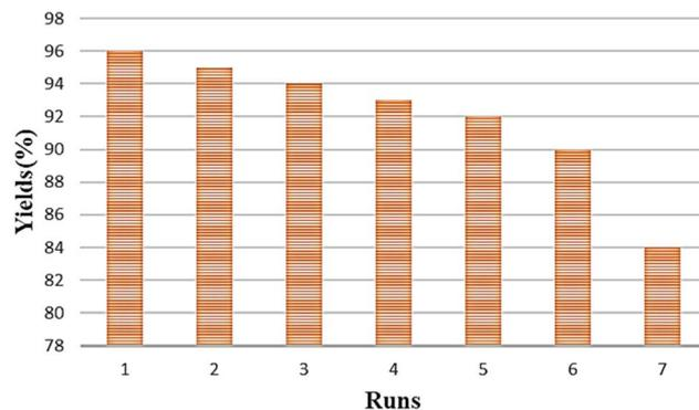
Fig. 10 Recyclability of the Cu-Amd-RGO in the synthesis of 5-substituted 1H-tetrazole.
