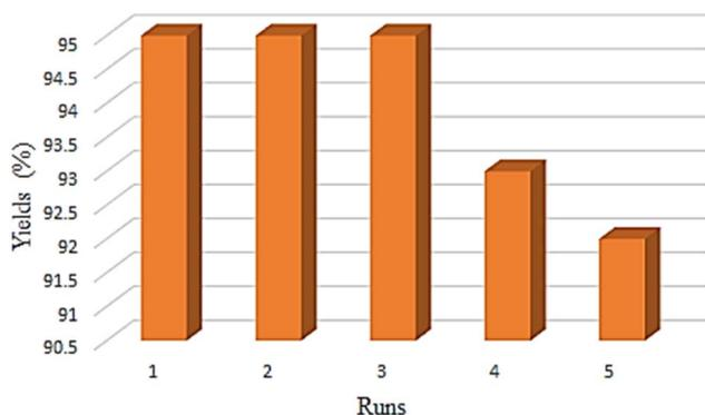
Fig. 9 Recyclability of the BNPs@SiO<sub>2</sub>-TPPTSA in the synthesis of 5-substituted 1H-tetrazole.
