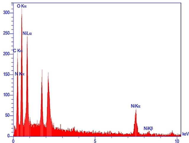
Fig. 3 EDX analysis of Ni-ascorbic acid MOF.
