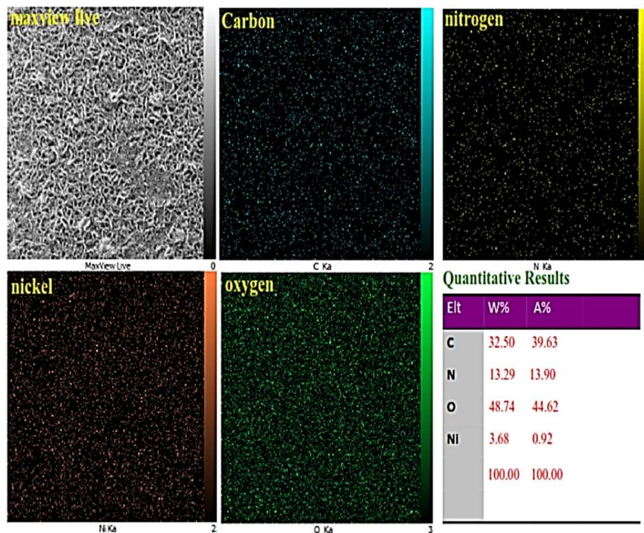
Fig. 4 Elemental mapping analysis of Ni-ascorbic acid MOF.
