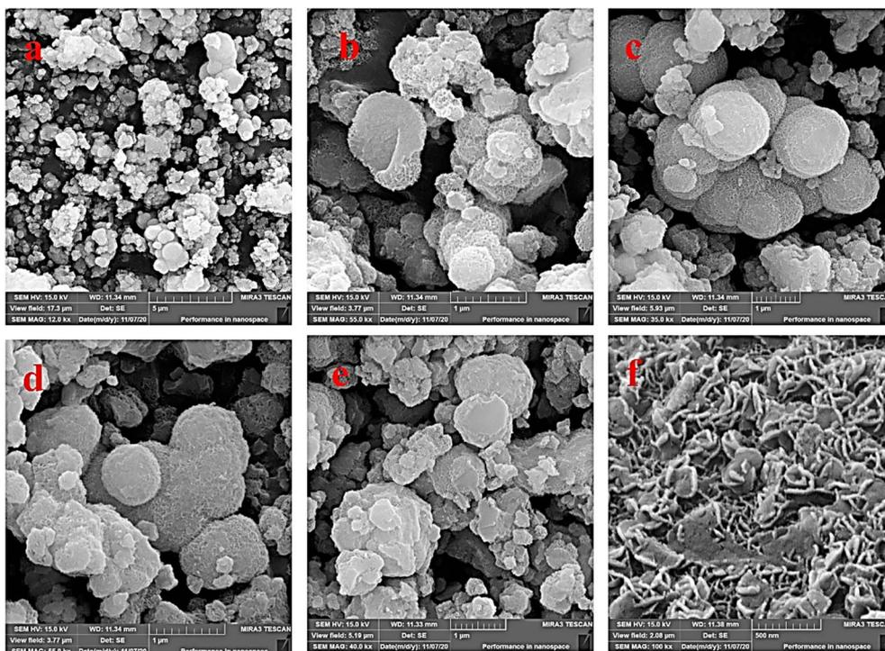
Fig. 5 (a–f) FE-SEM images of Ni-ascorbic acid MOF.
