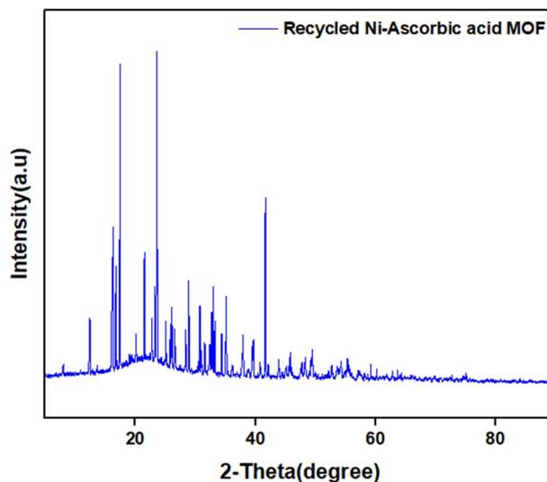
Fig. 12 XRD spectra of Ni-ascorbic acid MOF after the reaction.
