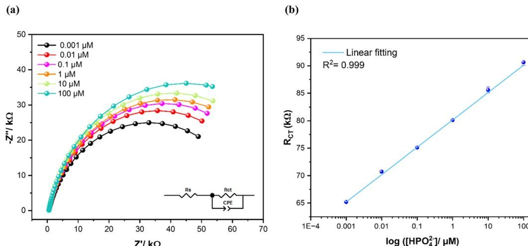
Fig. 7 (a) Electrochemical impedance spectroscopy responses as Nyquist plots of CuPc/MWCNTs/CSPE in different concentrations of phosphate in 25 mM of KHP KCl buffer at pH 7 and 50  $\text{mV s}^{-1}$  scan rate. The inset illustrates the electric equivalent circuit; (b) calibration curve of phosphate detection in the concentration range from 0.001  $\mu\text{M}$  to 100  $\mu\text{M}$ , error bars represent standard deviations of three independent measurements.
