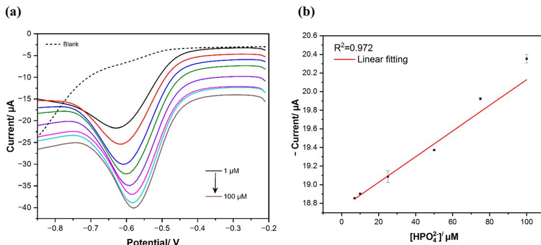
Fig. 6 (a) Square wave voltammograms responses of MWCNTs/CuPc/CSPE in different phosphate concentrations in 25 mM KHP buffer and 1 mM KCl buffer at pH 7 and 50 mV s<sup>-1</sup> scan rate; (b) calibration curve of phosphate determination in the concentration range of 10 to 100  $\mu\text{M}$  (error bars indicate standard deviations over three independent measurements).
