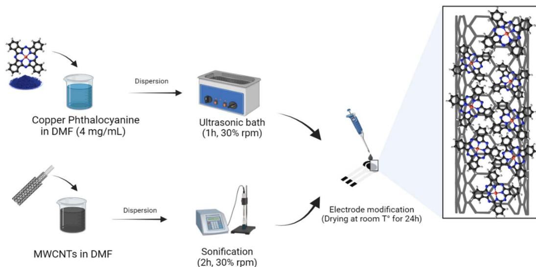
Fig. 1 Illustration of nanomaterials and electrode preparation steps.
