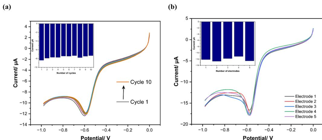
Fig. 9 (a) CV response of 15 cycles with same modified electrode, (b) CV of 5 different sensors response prepared under same experimental conditions.
