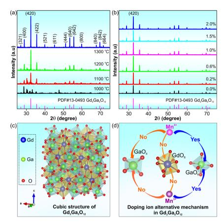
Fig. 1 XRD patterns of (a)  $Gd_3Ga_5O_{12}$ :0.2% Mn phosphors annealed at various temperatures and (b)  $Gd_3Ga_5O_{12}$ :x% Mn (x = 0.0-2.0) phosphors annealed at 1300 °C (c) cubic structure of the  $Gd_3Ga_5O_{12}$  lattice modeled using VESTA software and (d) preferred substitution of Mn<sup>3+</sup> and Mn<sup>4+</sup> ions for  $Ga^{3+}$  ions  $[GaO_6]$  sites in the  $Gd_3Ga_5O_{12}$  lattice.
