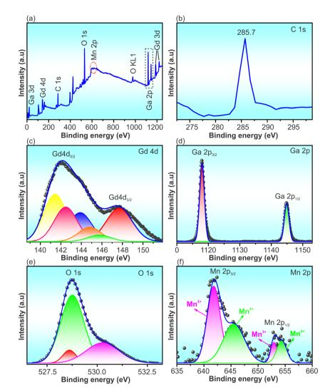
Fig. 5 XPS spectra of  $Gd_3Ga_5O_{12}$ : 0.2%Mn sample: (a) survey spectrum, (b) C 1s, (c) Gd 4d, (d) Ga 2p, (e) O 1s and (f) Mn 2p.
