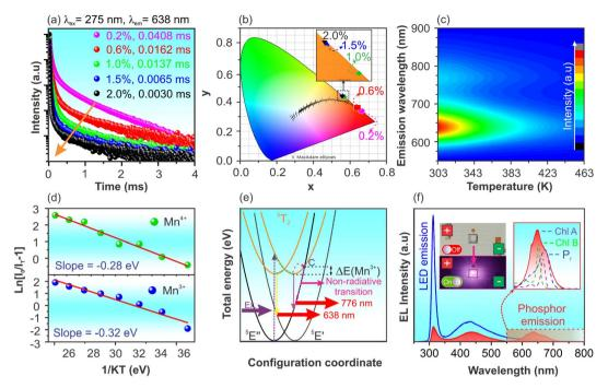
Fig. 8 (a) Lifetime curves for the 638 nm peak under 275 nm excitation, with the arrow indicating the increase of doping concentration; (b) CIE diagram of  $Gd_3Ga_5O_{12}$ : x% Mn (x = 0.2-2.0) annealed at 1300 °C in air for 5 h; (c) PL spectrum measured at temperatures in range of room temperature (300 K) to 463 K; (d) correlation between 1/kT and  $\ln(I_0/I_T-1)$ ; (e) schematic representation of the thermal quenching mechanism in  $Gd_3Ga_5O_{12}$ :Mn phosphor.
