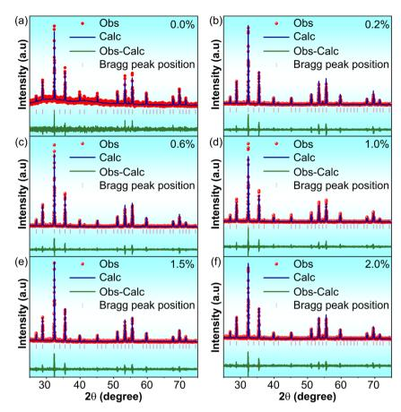
Fig. 2 Rietveld refinement for the  $Gd_3Ga_5O_{12}$ :x%Mn (x = 0.0-2.0) phosphors annealed at 1300 °C for 5 hours in air.
