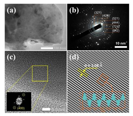
Fig. 3 (a) TEM image, (b) selected area electron diffraction (SAED) pattern, (c) high-resolution TEM (HRTEM) image and (d) IFFT images and corresponding lattice plane fringes of the  $Gd_3Ga_5O_{12}$ :0.2%Mn sample annealed at 1300 °C for 5 hours in air.
