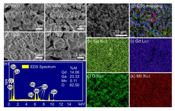
Fig. 4 (a-d) FESEM images of the  $Gd_3Ga_5O_{12}$ :0.2%Mn samples annealed at 1000–1300 °C. (e) EDS elements spectrum and (f) The scanned FESEM of EDS (g-k) EDS mapping spectra of the  $Gd_3Ga_5O_{12}$ :0.2%Mn sample annealed at 1300 °C.
