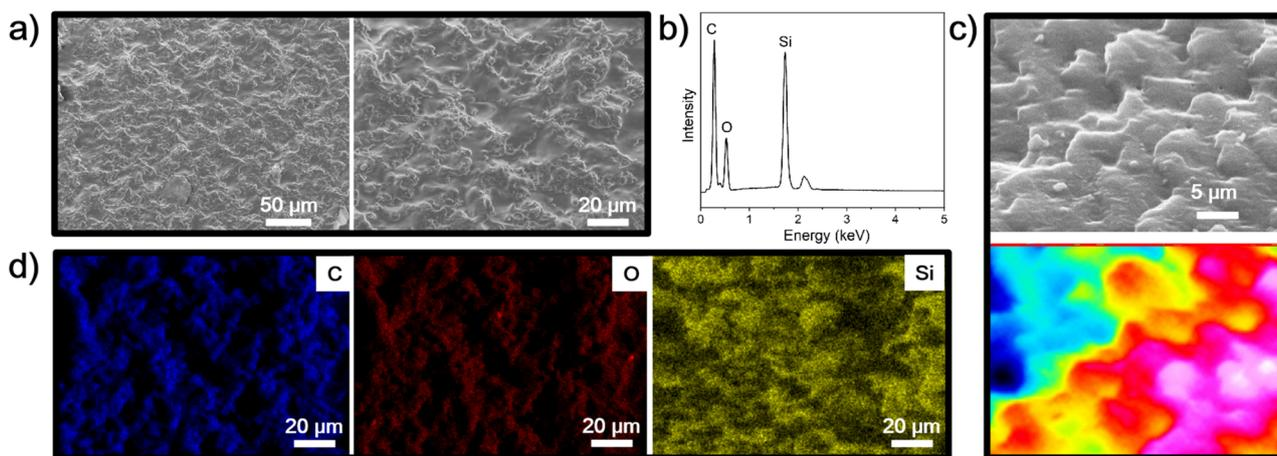
Fig. 5 SEM (a), EDS (b), 3D scanning of SEM (c) and element mapping (d) of PUA-Si 7000 Da.
