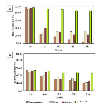
Fig. 12 Performance of various regeneration materials of organoclay—activated carbon for (a) PRD removal, (b) SAL.
