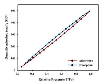
Fig. 7 The adsorption–desorption isotherms of N<sub>2</sub> for OC/AC at 77 K.
