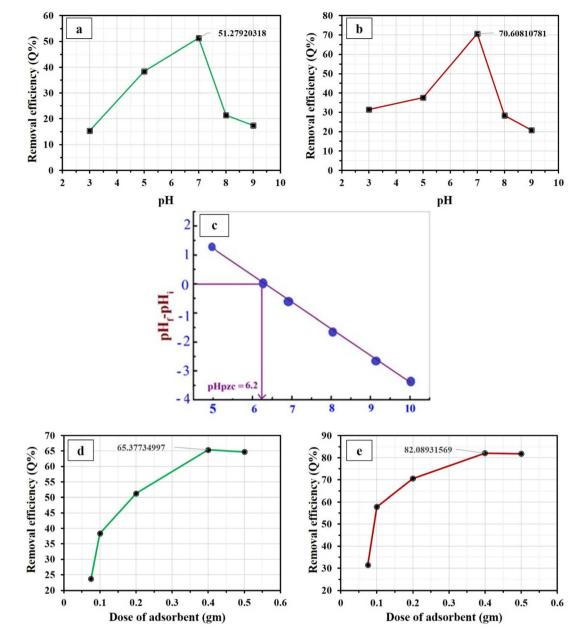
Fig. 8 (a and b) Effect of pH on the adsorption of (a) SAL and (b) PRD, while (c) PZC of OC/AC, (d and e) effect of dose of adsorbent on the removal efficiency of (d) SAL, (e) PRD.
