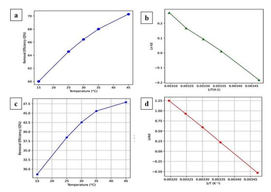
Fig. 9 (a) The effect of temperature on the removal efficiency to remove SAL; and (b) a plot of  $\ln K_d$  against 1/T(K-1) for SAL, (c) The effect of temperature on the removal efficiency to remove PRD and (d) a plot of  $\ln K_d$  against 1/T(K-1) for PRD.
