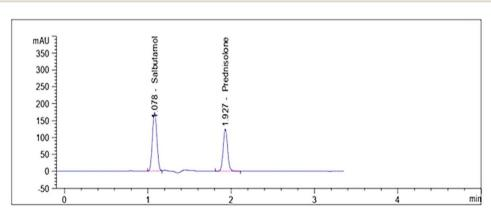
Fig. 2 HPLC chromatograms of SAL and PRD recorded at the optimum wavelength of 214 nm.
