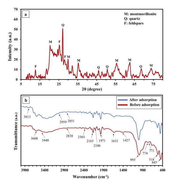
Fig. 5 (a) XRD-analysis of OC/AC composite and (b) FTIR spectrum of OC/AC before and after adsorption.
