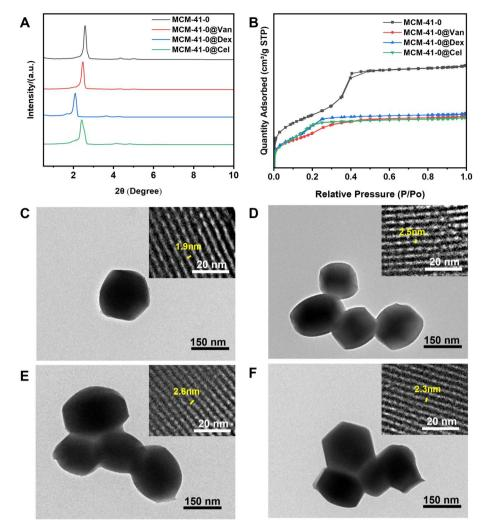
Fig. 1 (A) XRD patterns of MCM-41-0, MCM-41-0@Van, MCM-41-0@Dex and MCM-41-0@Cel, (B)  $N_2$  adsorption—desorption isotherms of MCM-41-0, MCM-41-0@Van, MCM-41-0@Dex and MCM-41-0@Cel, TEM image of (C) MCM-41-0, (D) MCM-41-0@Van, (E) MCM-41-0@Dex, (F) MCM-41-0@Cel.
