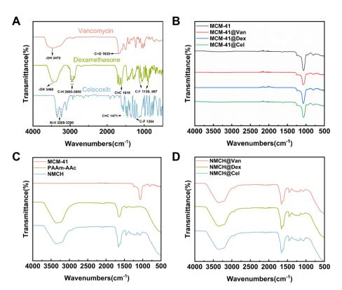
Fig. 2 FT-IR spectra of (A) three kinds of medicines with featured absorptions, (B) MCM-41-0 loading Van, Dex and Cel., (C) MCM-41, PAAm-AAc and NMCH, (D) NMCH containing different medicines.
