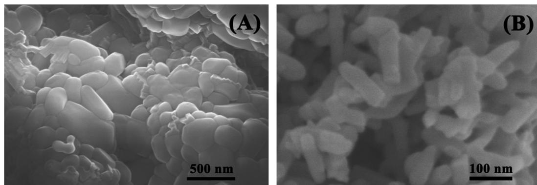
Fig. 16 SEM images of the synthetic crystals aged at 60 °C for 24 hours (A) and 48 hours (B).<sup>55</sup>
