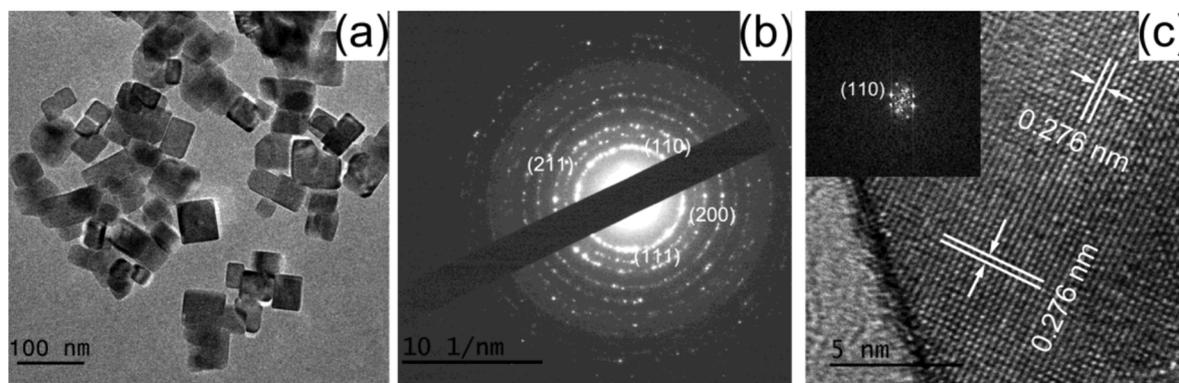
Fig. 7 TEM micrographs of S1-20: (a) 100 nm, (b) SAED, (c) HRTEM.<sup>40</sup>
