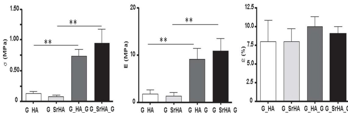
Fig. 22 Mean values of collapse stress ( $\sigma$ ), linear elastic modulus ( $E$ ), and strain ( $\epsilon$ %) of the different scaffolds. Each value is the mean of six determinations and is reported with its standard deviation (\*\* $p < 0.001$ ). Stress: \*\*G\_HA versus G\_HA\_G; G\_SrHA versus G\_SrHA\_G. Elastic modulus: \*\*G\_HA versus G\_HA\_G; G\_SrHA versus G\_SrHA\_G.<sup>145</sup>
