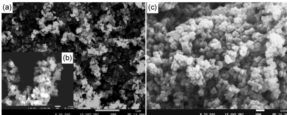
Fig. 5 SEM micrographs of the SrTiO<sub>3</sub> nanoparticles: (a and b) S1-40, (c) S2-40.<sup>40</sup>
