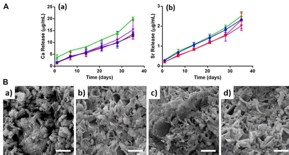
Fig. 33 (A) Ion releases up to 35 days: (a) calcium, (b) strontium. SrCPC (blue), SrCPC\_NP (red), SrCPC\_TC (green), SrCPC\_NP-TC (violet); (B) SEM micrographs of cements: CPC (a), CPC\_TC (b), CPC\_NP (c), CPC\_NP-TC (d). Scale bar = 5 µm.<sup>195</sup>
