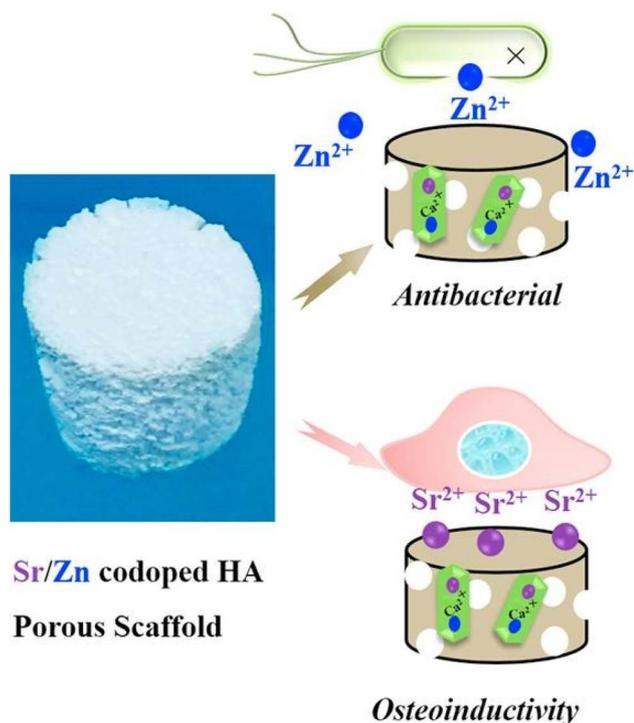
Fig. 21 Sr/Zn codoped hydroxyapatite (HA) porous scaffold: enhanced antibacterial properties and osteoinductive potential for bone regeneration applications.<sup>144</sup>
