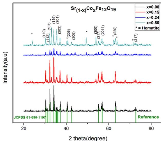
Fig. 14 XRD pattern of  $\text{Sr}_{1-x}\text{Co}_x\text{Fe}_{12}\text{O}_{19}$ .<sup>52</sup>
