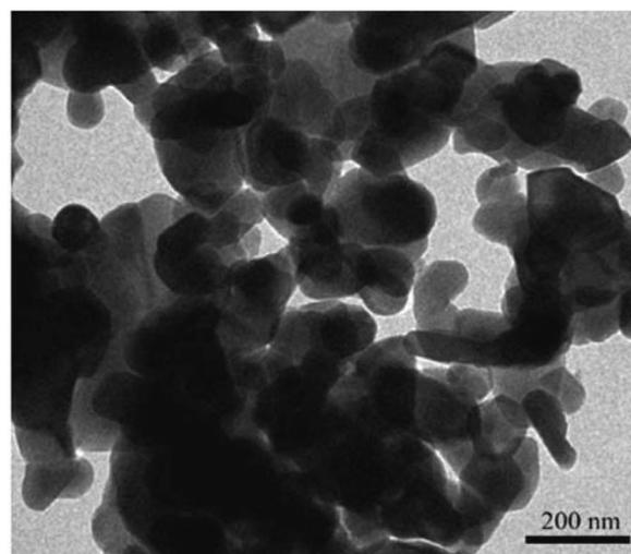
Fig. 1 Micrographs of strontium hexaferrite obtained by transmission electron microscopy (TEM) of the SGP sample.<sup>31</sup>
