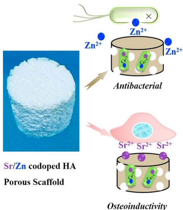
Fig. 21 Sr/Zn codoped hydroxyapatite (HA) porous scaffold: enhanced antibacterial properties and osteoinductive potential for bone regeneration applications. 144
