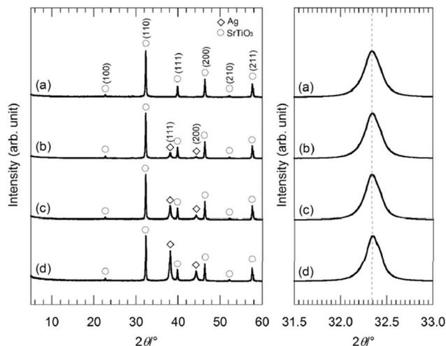
**Fig. 10** (Left) XRD patterns of the hybrid particles synthesized from the precursor gels with molar ratios of (a) Ag : Sr : Ti = 0 : 4 : 4; (b) 1 : 4 : 4; (c) 2 : 4 : 4; and (d) 4 : 4 : 4 by the hydrothermal treatment at 230 °C for 6 h in Sr(OH)<sub>2</sub> aqueous solutions; (Right) XRD peaks of the hybrid particles indexed as (110) of SrTiO<sub>3</sub> in the  $2\theta$  range of 31.5–33.0°.<sup>21</sup>
