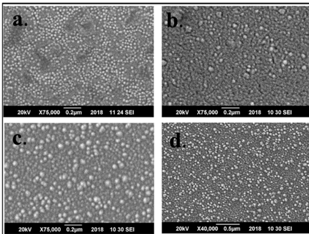
Fig. 15 Morphological analysis using SEM for  $\text{Sr}_{1-x}\text{Co}_x\text{Fe}_{12}\text{O}_{19}$  (a)  $x = 0$ , (b)  $x = 0.15$ , (c)  $x = 0.24$ , and (d)  $x = 0.5$ .<sup>52</sup>
