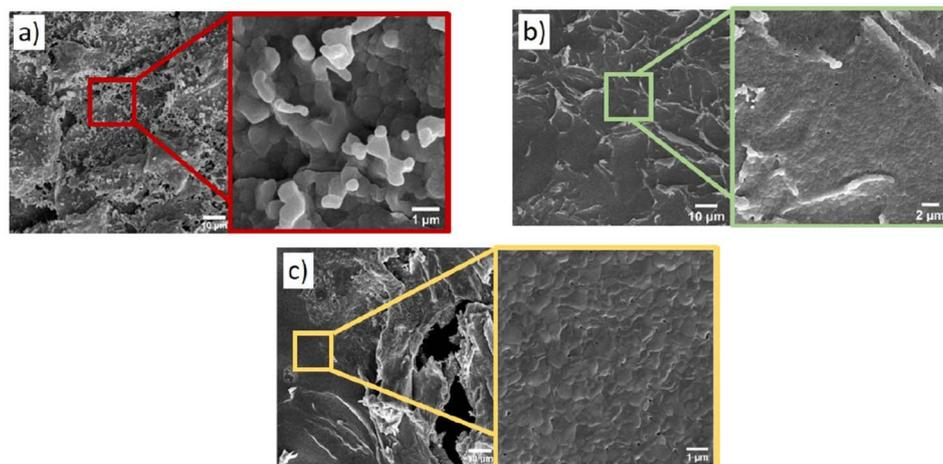
**Fig. 11** SEM micrographs of surface Al<sub>2</sub>O<sub>3</sub>/SrCO<sub>3</sub> xerogels with the 1.0 Sr molar ratio annealed at: (a) 1000 °C (1273 K), (b) 1150 °C (1423 K), and (c) 1300 °C (1573 K).<sup>51</sup>
