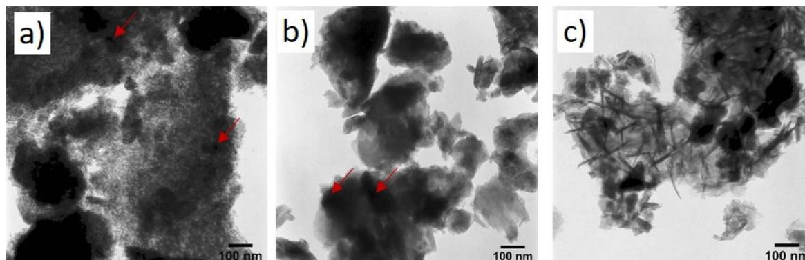
Fig. 13 TEM images of  $\text{Al}_2\text{O}_3/\text{SrCO}_3$  sol-gel incorporated with Pt after annealing at 500 °C, showing molar ratios of: (a) Sr : 0.1 Pt, (b) Sr : 0.25 Pt, and (c) Sr : 0.5 Pt.<sup>51</sup>
