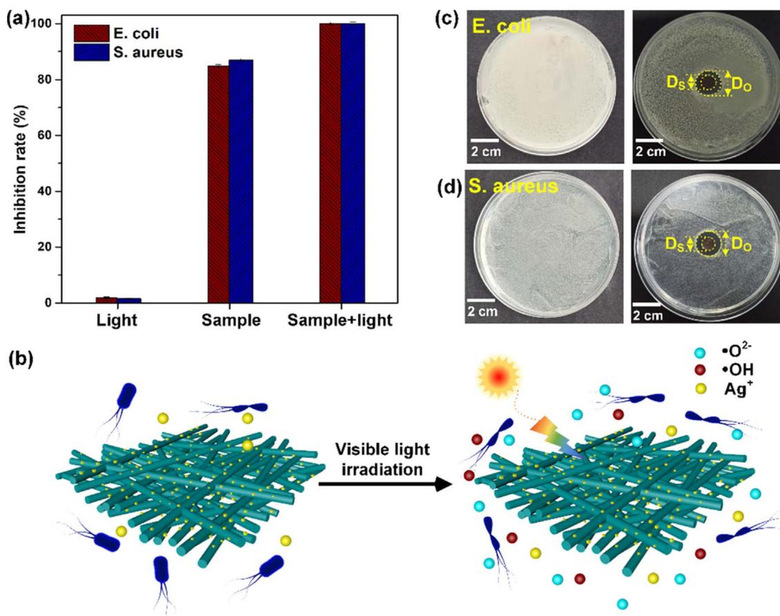
Fig. 32 (a) The inhibition rate of AZSTO nanofibrous membranes against *E. coli* and *S. aureus* under different conditions. (b) Schematic illustrating the disinfection mechanism of AZSTO nanofibrous membranes. Optical profiles showing the inhibition zone test against (c) *E. coli* and (d) *S. aureus*: unprocessed (left) and treated with AZSTO nanofibrous membranes under visible-light irradiation (right).<sup>193</sup>
