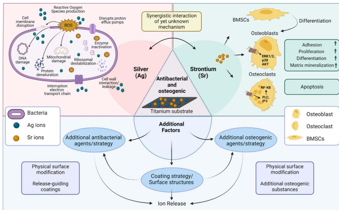
Fig. 24 Schematic illustration of possible mechanisms related to antibacterial/osteogenic titanium surfaces in the included studies. Abbreviations: BMSCs, bone marrow stromal cells; ERK1/2, extracellular signal-regulated kinases 1/2; NF-KB, nuclear factor *k*-light-chain-enhancer of activated B cells.<sup>60</sup>
