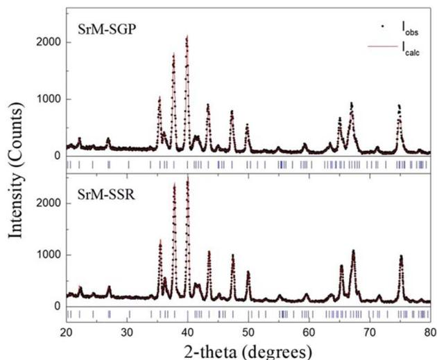
Fig. 2 X-ray patterns and Rietveld refinement adjusts for the strontium hexaferrite prepared by the sol-gel Pechini (SGP) method and the solid-state reaction (SSR) method.<sup>31</sup>
