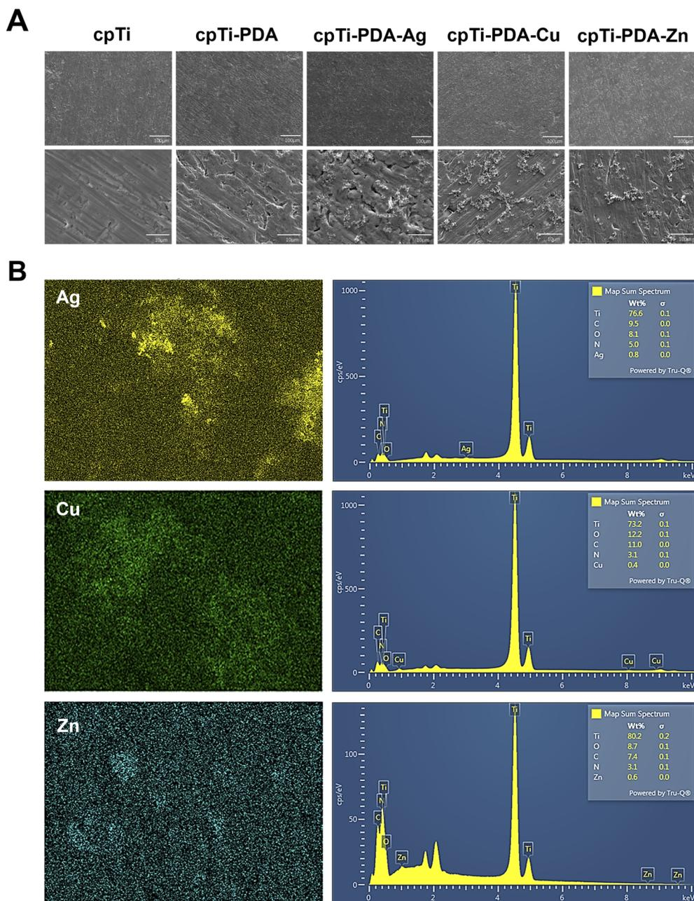
**Fig. 1** Surface microstructures of the coatings. (A) Surface microstructures of different specimen surfaces. (B) Energy-dispersive X-ray mapping of the cpTi-PDA-Ag, cpTi-PDA-Cu and cpTi-PDA-Zn surface.
