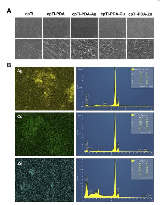
Fig. 1 Surface microstructures of the coatings. (A) Surface microstructures of different specimen surfaces. (B) Energy-dispersive X-ray mapping of the cpTi-PDA-Aq, cpTi-PDA-Cu and cpTi-PDA-Zn surface.
