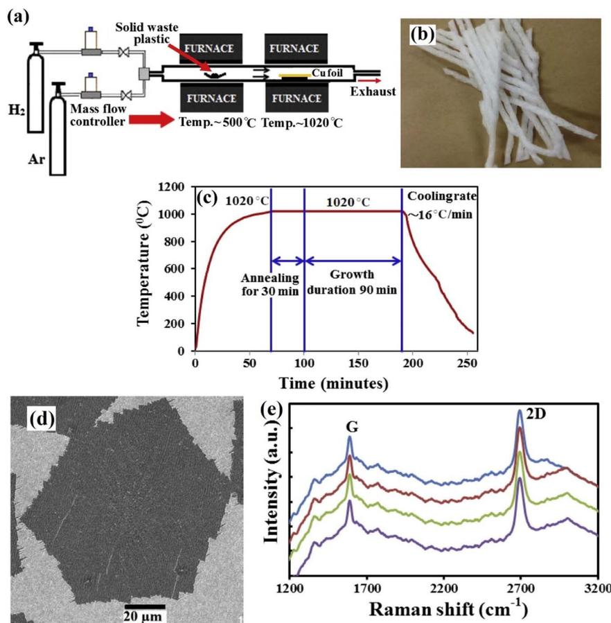
Fig. 16 (a) Schematic of CVD for the preparation of graphene sheets on Cu foil; (b) fruit protective foam plastic waste; (c) the graphene development process's heating, annealing, growth time, and cooling rate; (d) TEM images of individual graphene crystals after growing for 90 minutes; and (e) Raman spectra of graphene films. Figure has been reproduced from ref. 124. Copyright 2014, Elsevier.
