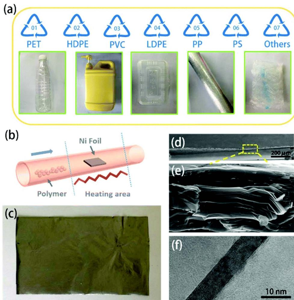
Fig. 17 (a) Various plastic types for experimental, (b) solid-state CVD system, (c) image of one large graphene foil  $17 \times 10 \text{ cm}^2$ . (d and e) SEM images of the graphene foil edge, and (f) cross-sectional TEM images with clear lattice spacing. Figure has been reproduced with permission from ref. 125. Copyright 2017, Royal Society of Chemistry.
