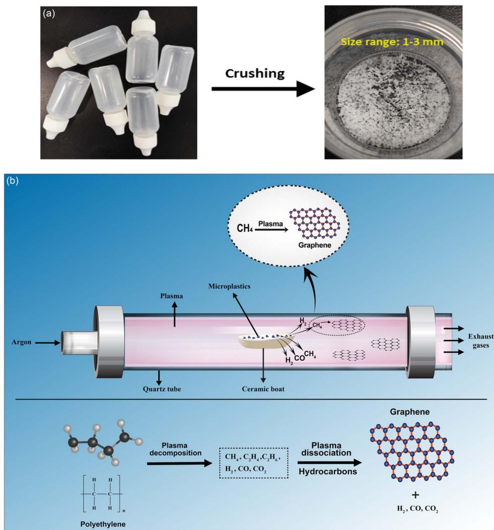
Fig. 18 (a) Illustration showing dropper bottles sliced into tiny plastic particles ranging in size from 1 to 3 mm. (b) A graphical representation of the APMP technique used to create graphene from PE microplastics. Figure has been reproduced ref. 129. Copyright 2024, Wiley.
