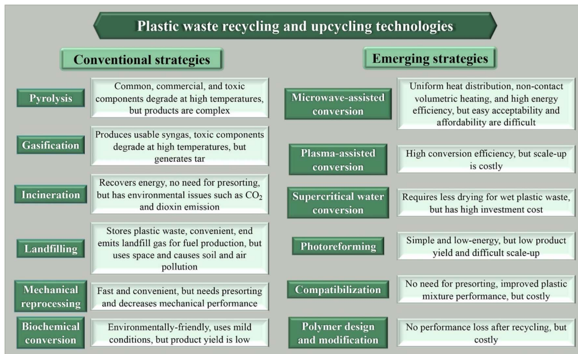
Fig. 20 An analysis of the main traditional and new approaches for the reuse and recycling of plastic waste. Figure has been reproduced with permission from ref. 135. Copyright 2022, Elsevier.
