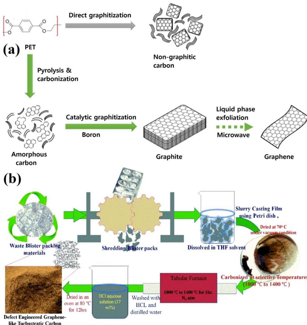
Fig. 15 (a) Diagram for turning PET plastic into graphite and graphene.<sup>119</sup> (b) Illustration of the turbostratic carbon produced via a carbonization process from blister packs.<sup>120</sup> Figure (a) has been reproduced with permission from ref. 119, copyright 2020, Elsevier. Figure (b) has been reproduced from ref. 120. Copyright 2022, Royal Society of Chemistry.
