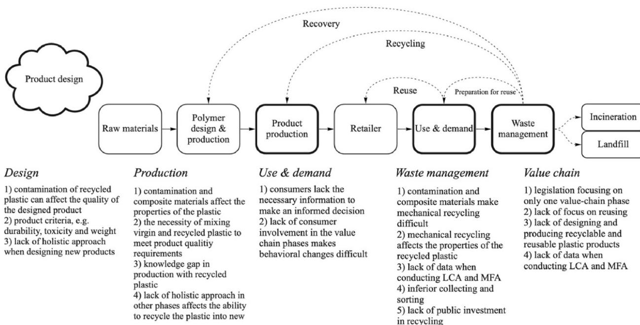
Fig. 19 From the manufacture of plastic to the disposal of plastic waste, every stage of the value chain represents tremendous challenges. Figure has been reproduced with permission from ref. 133. Copyright 2022, Elsevier.
