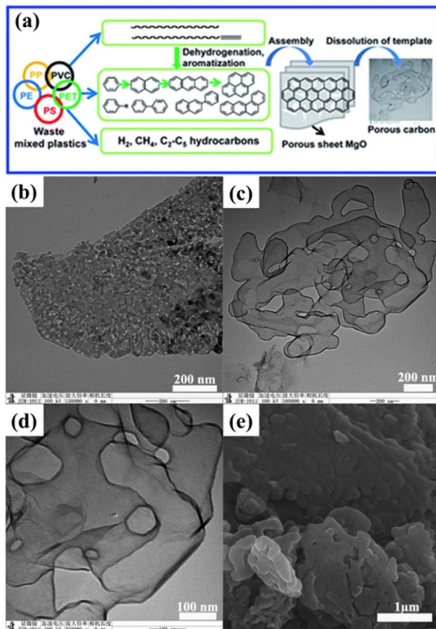
Fig. 14 (a) Schematic of the preparation of porous carbon sheets, and morphology determined from (b–d) TEM images and (e) SEM images. Figure has been reproduced with permission from ref. 118. Copyright 2018, Royal Society of Chemistry.
