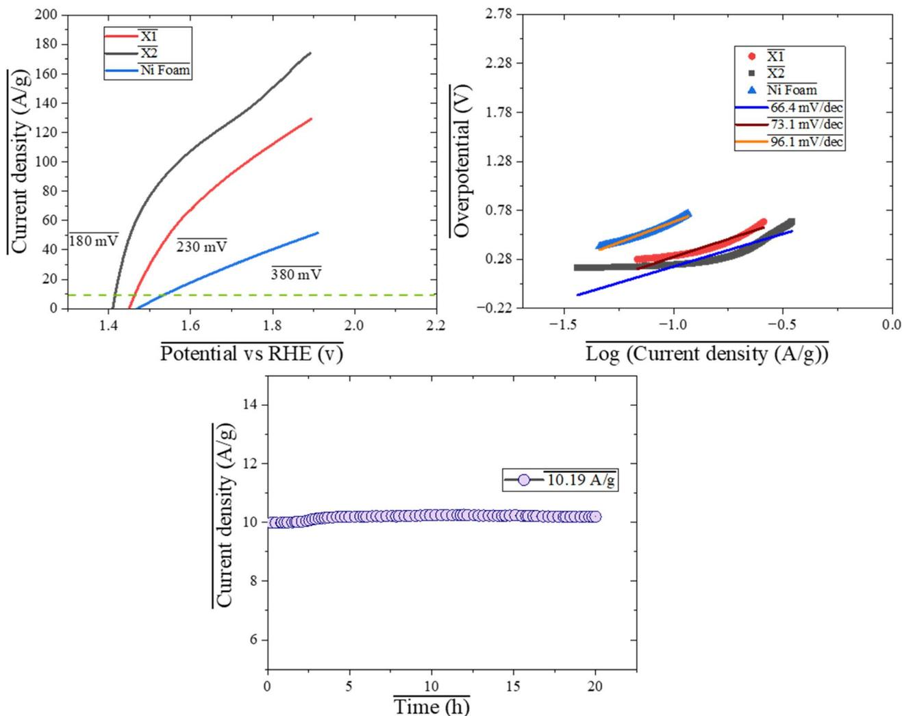
Fig. 5 (a) OER polarization curves of X1, X2 and bare Ni foam (b) Tafel slope, (c) stability test outcome of X2 while being operated at 10 A g<sup>-1</sup>.
