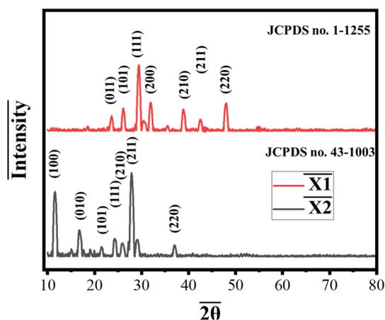
Fig. 1 XRD characterization of the synthesized Co-MOFs, X1 and X2.
