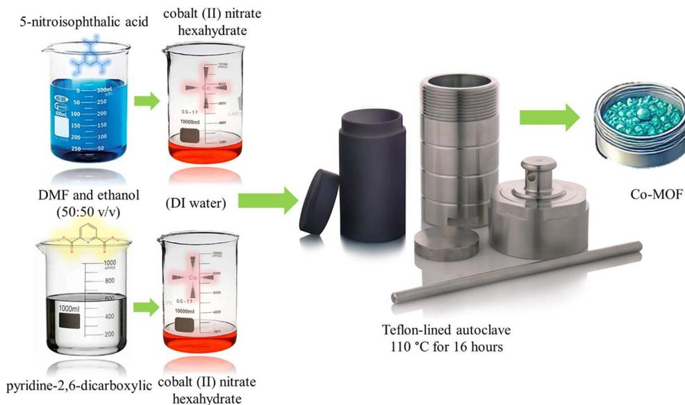
Scheme 1 Schematic illustration of hydrothermal synthesis process adopted.
