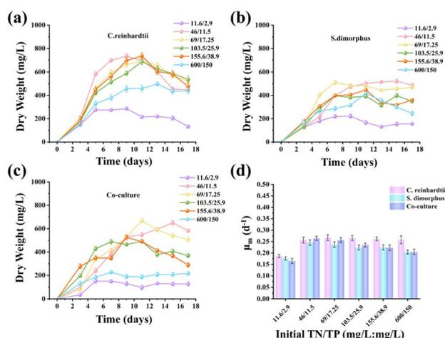
**Fig. 1** Growth characteristics and nutrient removal performance of *C. reinhardtii*, *S. dimorphus*, and their co-culture under different N/P concentrations. (a) Biomass accumulation of *C. reinhardtii*; (b) biomass accumulation of *S. dimorphus*; (c) biomass accumulation of co-culture; (d) specific growth rates. All values are presented as means  $\pm$  standard deviation ( $n = 3$ ).
