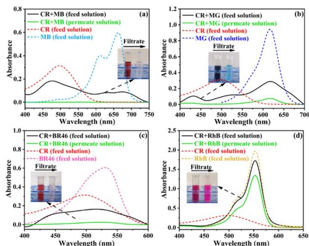
Fig. 11 The rejection performance of M1 membrane for different mixed dyes: (a) CR + MB, (b) CR + MG, (c) CR + BR46, (d) CR + RhB.
