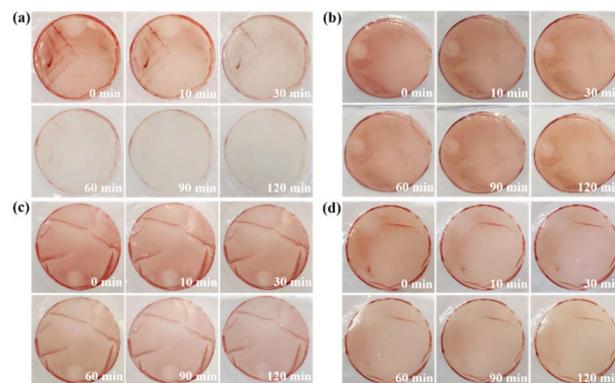
Fig. 13 Photographs of the color changes of polluted (a–c) M1 membrane and (d) M0 membrane with reaction time under different conditions: (a) light and H<sub>2</sub>O<sub>2</sub>, (b) H<sub>2</sub>O<sub>2</sub>, (c) light, (d) light and H<sub>2</sub>O<sub>2</sub>.
