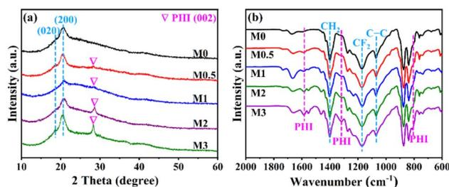
Fig. 3 (a) XRD patterns and (b) FTIR spectra of pure PVDF and PHI/PVDF membranes.
