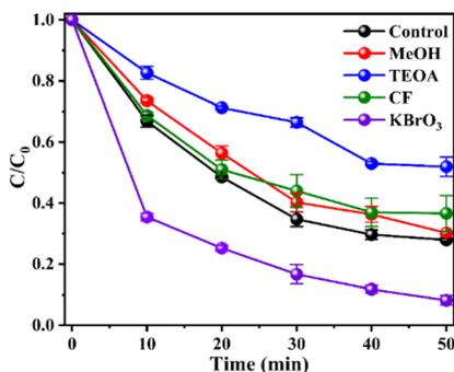
Fig. 15 Effects of different scavengers on the catalytic degradation of CR by PHI. Experimental conditions:  $[\text{PHI}] = 1 \text{ g L}^{-1}$ ,  $[\text{H}_2\text{O}_2] = 80 \text{ mM}$ ,  $[\text{CR}] = 20 \text{ mg L}^{-1}$ ,  $T = 30 \text{ }^\circ\text{C}$ .
