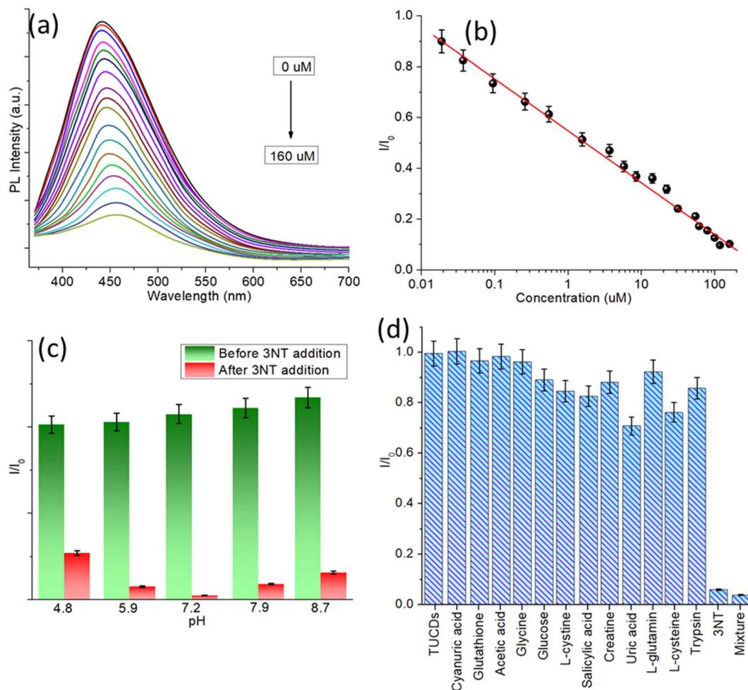
Fig. 7 (a) PL spectra of TUCDs with different concentrations of 3NT (b) change of PL intensity signal with 3NT concentration (c) change of PL intensity signal in different pH with and without 3NT concentration (d) selectivity analysis of TUCDs against different physiological solutions showing fluctuations of PL intensities.
