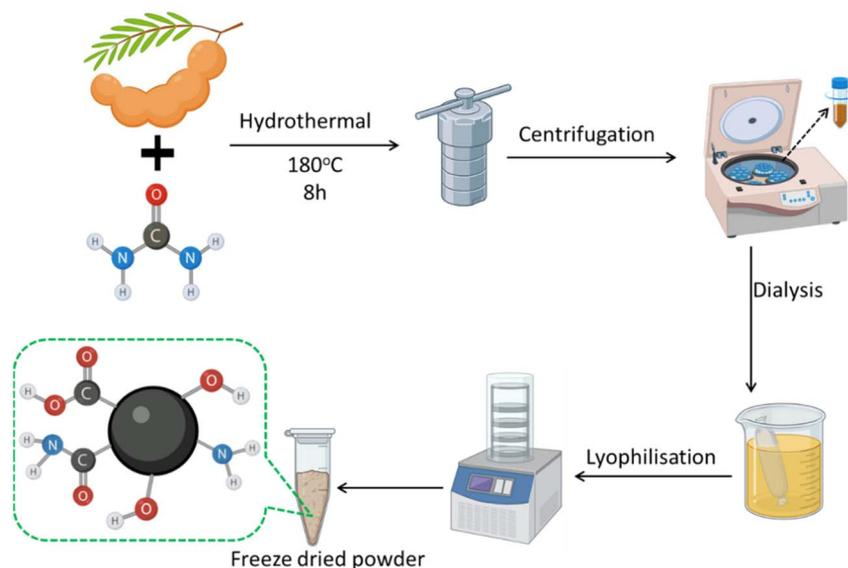
Fig. 1 Schematic representation of synthesis of TUCDs.
