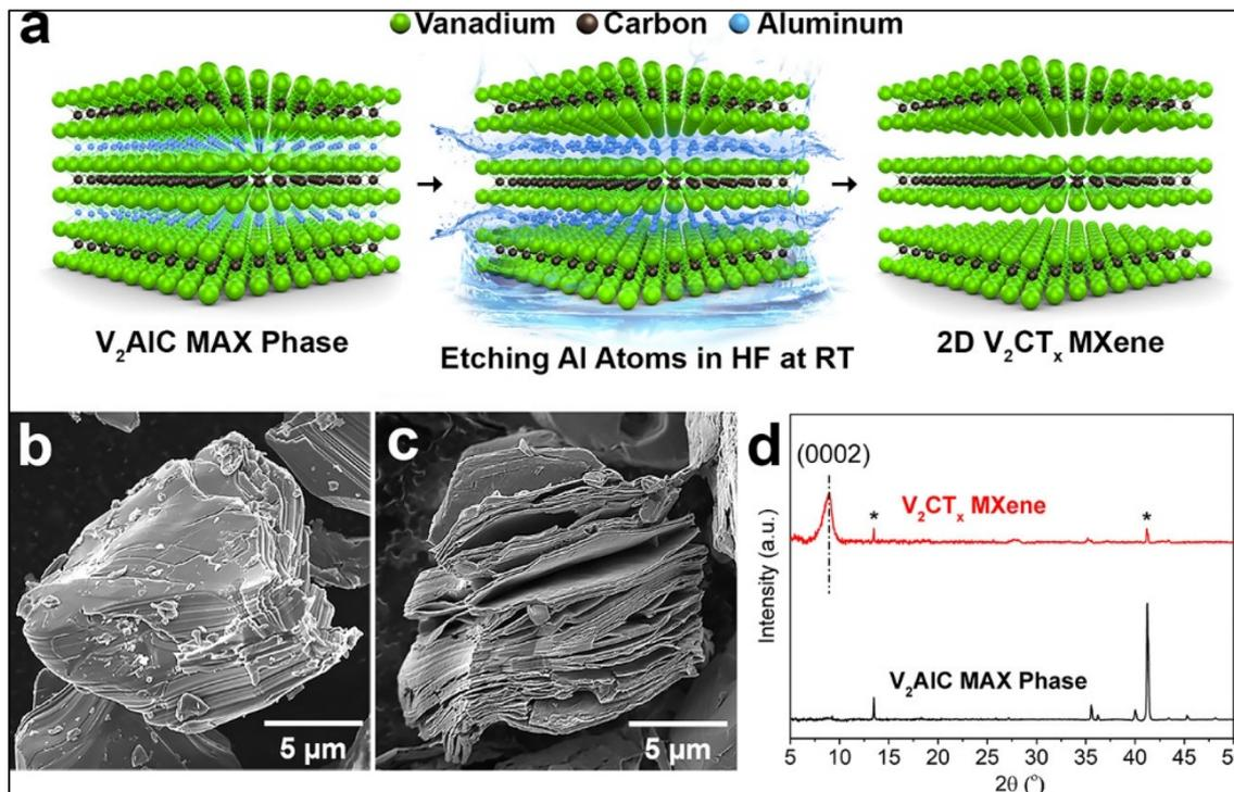
Fig. 1 (a) Schematic representation of  $V_2CT_x$  synthesis from  $V_2AlC$ ; SEM images of (b)  $V_2AlC$  phase and (c)  $V_2CT_x$ . (d) XRD patterns of  $V_2AlC$  and  $V_2CT_x$ , (\*) denotes residual  $V_2AlC$  phase.<sup>27</sup>
