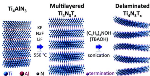
Fig. 3 Schematic of molten salt synthesis of  $\text{Ti}_4\text{N}_3\text{T}_x$  from  $\text{Ti}_4\text{AlN}_3$  at  $550^\circ\text{C}$  and delamination by TBAOH.
