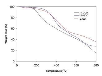
Fig. 7 TGA thermograms of pristine N-GQDs, Si-GQD and f-GQD.
