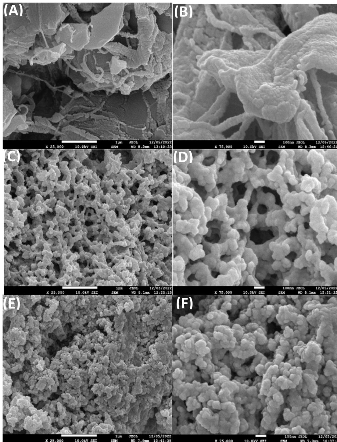
Fig. 4 SEM images of pristine N-GQDs (A and B), Si-GQD (C and D) and f-GQD (E and F) with different magnification.
