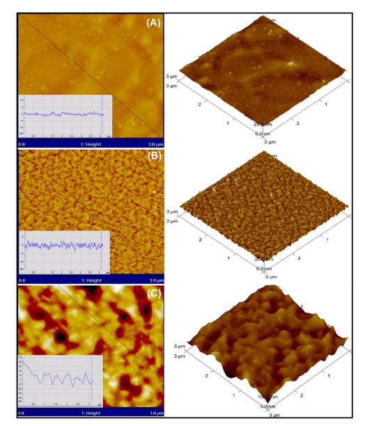
Fig. 6 AFM images of pristine (A) N-GQDs, (B) Si-GQD, and (C) f-GQD.
