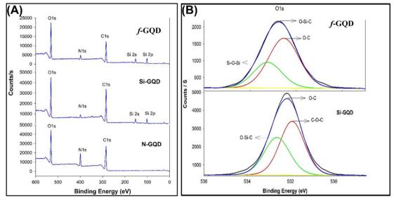
Fig. 3 XPS spectrum of (A) pristine N-GQDs, Si-GQD, and f-GQD; (B) deconvoluted oxygen peaks of Si-GQD and f-GQD.
