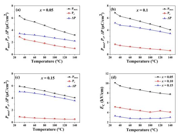
Fig. 6 Thermal variation of  $P_{\text{max}}$ ,  $P_{\text{r}}$  and  $\Delta P = (P_{\text{max}} - P_{\text{r}})$ , measured under an electric field of 30 kV cm<sup>-1</sup> for (BZT-Pr-xNBT) samples with (a) x = 10.05, (b) x = 0.10 and (c) x = 0.15. In addition, panel (d) presents a comparison of the coercive field ( $E_C$ )
