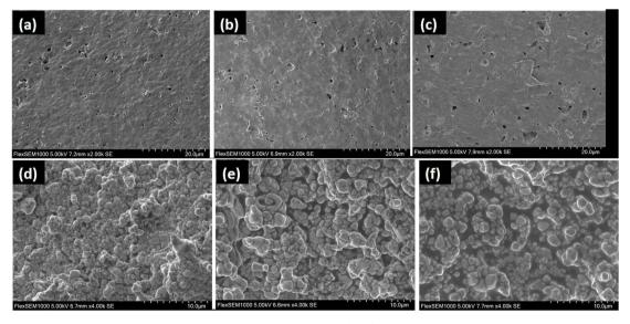
Fig. 2 Surface morphology and grain size analysis of BZT-Pr-xNBT samples: (a-c) surface morphology for x = 0.05, 0.10, and 0.15; (d-f) grain observation on fractured samples for x = 0.05, 0.10, and 0.15.
