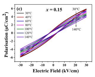
Fig. 5 Polarization *versus* electric field (P-E) hysteresis loops for BZT-Pr-xNBT samples as a function of temperature under a constant electric field of 30 kV cm<sup>-1</sup> for (a) x = 0.05, (b) x = 0.10 and (c) x = 0.15.
