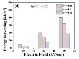
Fig. 11 Energy conversion *versus* electric field plots for (BZT-Pr-xNBT) samples with NBT content of (a) x = 0.05, (b) x = 0.10 and (c) x = 0.15 at  $E_L = 0$  kV cm<sup>-1</sup>. In addition, panel (d) compares the energy conversion capacity across the studied compositions.
