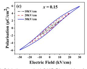
Fig. 4 Polarization *versus* electric field (P-E) hysteresis loops for BZT-Pr-xNBT samples at constant temperature (30 °C) for (a) x=0.05, (b) x=0.10, and (c) x=0.15, measured under varying electric field magnitudes.
