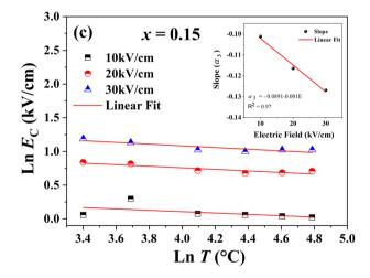
Fig. 8 Logarithmic plots of coercive field ( $E_{\rm C}$ ) versus temperature (T) under varying electric fields for BZT-Pr-xNBT ceramics with (a) x=0.05, (b) x=0.10 and (c) x=0.15 and the insets show the slope variations with electric field.
