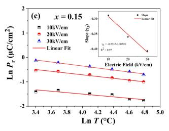
Fig. 9 Logarithmic plots of remnant polarization ( $P_r$ ) versus temperature (T) under varying electric fields for BZT-Pr-xNBT ceramics with (a) x=0.05, (b) x=0.10 and (c) x=0.15 and the insets show the slope variations with electric field.
